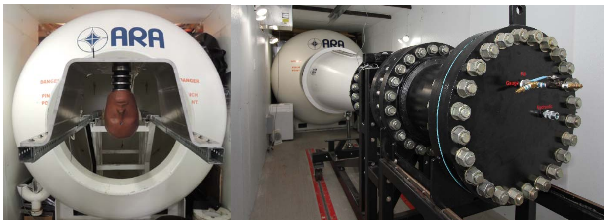
Figure 13: ARA's Mobile Shock Tube is capable of exposing a target to incident pressures of 168 dBP to 209 dBP.
