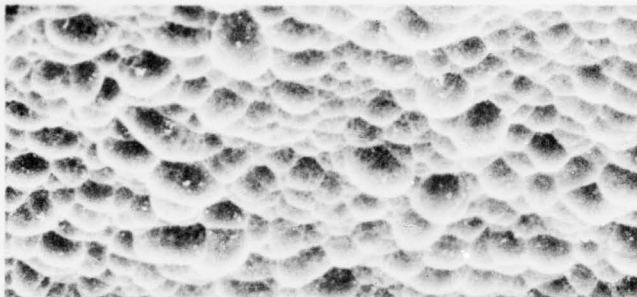
Ground with 22 μm Al 2 O 3 and 0.5-hour HF etch
