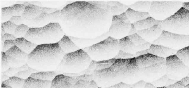
Ground with 22 μm Al 2 O 3 and 2.0-hour HF etch
