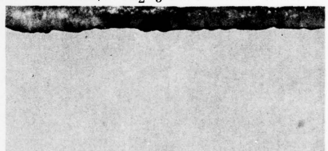
Ground with 9 μm Al 2 O 3 and 2.0-hour HF etch
