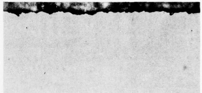
Ground with 9 μm Al 2 O 3 and 0.5-hour HF etch
