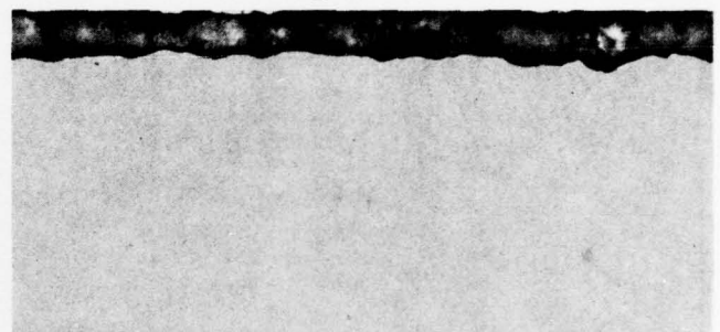
Ground with 9 μm Al 2 O 3 and 1.0-hour HF etch
