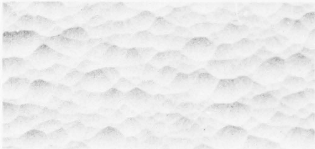
Ground with 3 \mu\text{m} \text{Al}_2\text{O}_3 and 2.5-hour HF etch
