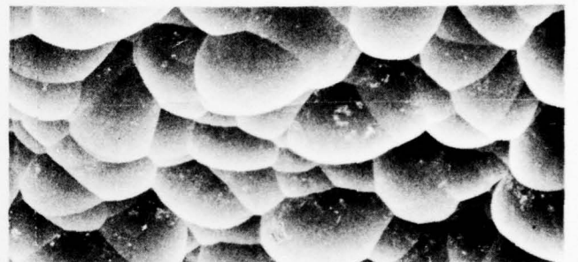
Ground with 177 μm SiC and 1.0-hour HF etch
