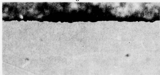
Ground with 3 μm Al 2 O 3 and 2.5-hour HF etch
