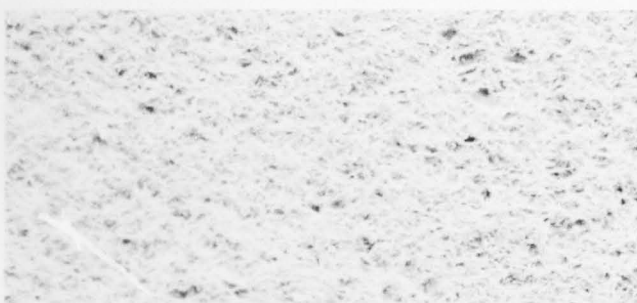
Ground with 22 μm Al 2 O 3 , no etching
