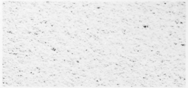
Ground with 9 \mu\text{m} \text{Al}_2\text{O}_3 , no etching
