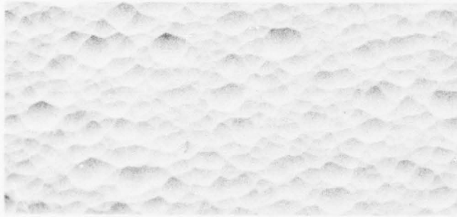
Ground with 3 \mu\text{m} \text{Al}_2\text{O}_3 and 1.0-hour HF etch
