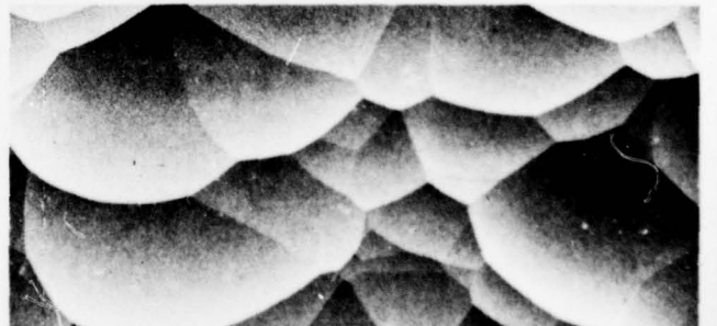
Ground with 177 μm SiC and 2.5-hour HF etch
