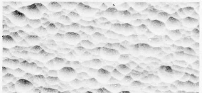
Ground with 9 \mu\text{m} \text{Al}_2\text{O}_3 and 1.0-hour HF etch
