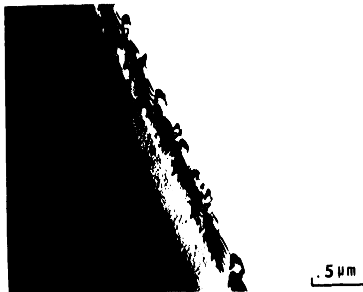
b. Typical Grain Boundary MC Precipitates
