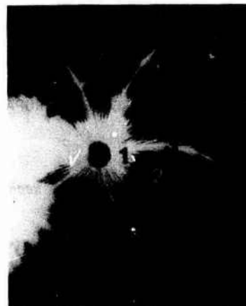
Fig. 2 - Photographic electric figure of a gliding spark of negative polarity 1 - Polar pre-discharge 2 - Spark channel 3 - Gliding pre-discharge
