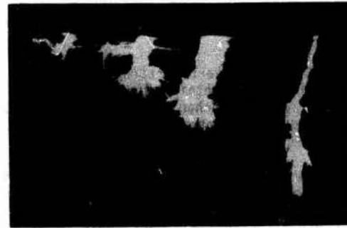
Figure 4 : I.C. streak cameragram of a negative discharge corresponding to T_{cr} < T_{cr.crit} . D = 7 m.
