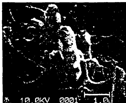
Figure 5. A SEM micrograph taken in the Auger microprobe of the fracture surface of a whisker SiC/Al composite.
