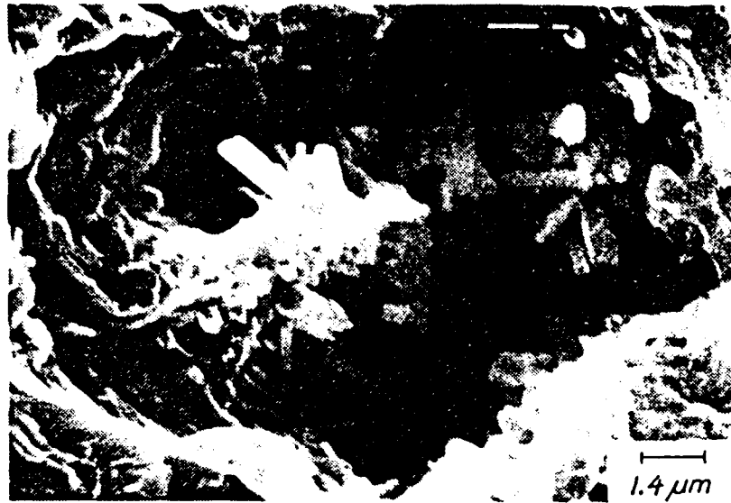
Figure 9 - Cluster of whiskers observed on the fracture surface of Silag 6061 Al/SiCw - 5 V% tested in annealed condition.
