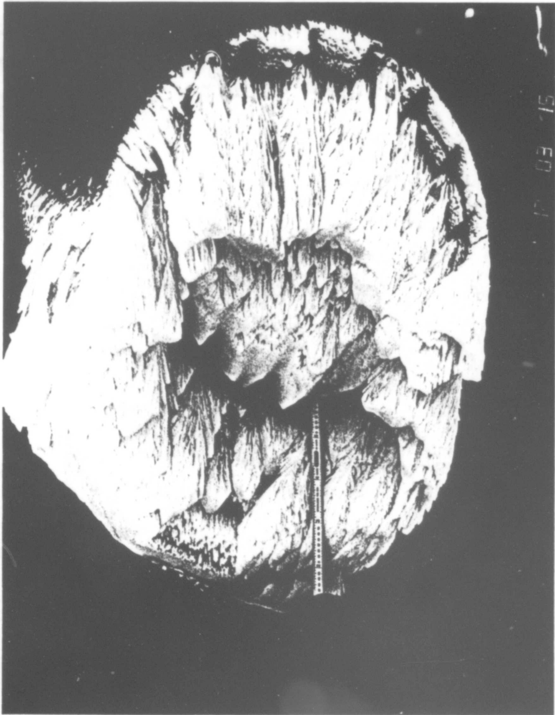
Figure H-11. AN/ALQ - 156 Antenna Accumulation Artificial Icing - .52 gm/m 3 LWC, -15.0 °C OAT, 60 min
