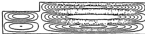
Fig.3 An example of a TE 02 /TE 03 complex cavity
