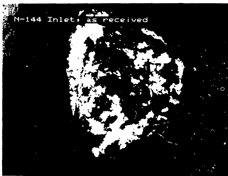
Figure 4. Backscattered Electron Image (BEI) of an ASC-TEDA Carbon Granule from the Filter Inlet following Weathering.
