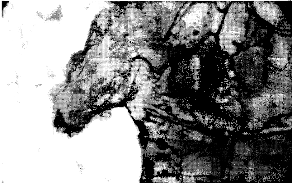
Figure 5-107. Cr 2 C 3 Plasma-Sprayed Coating, Synthetic Oil, Worn Near T.R.R., 266 RPM, 70 Lbf/In Load, 427 C, Normal Force 19 lbf, 2-Hour Test, More Film than Cr 2 O 3 for Same Condition, Objective Lens: 25/0.50, Photo Lens: X 10, Magnification: X 430
