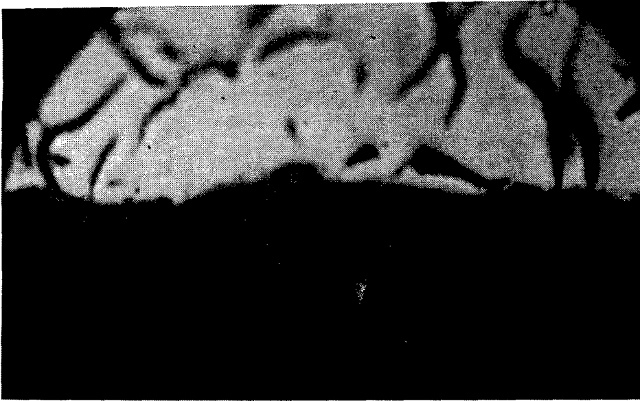
Figure 5-98. Cr 2 O 3 -Dipped Coating, Unworn, Surface Layer Thickness 0.035 mm, 0.1 Kg Load Vickers Test, Small Cracks at Left Corner, Objective Lens: 50/0.85, Photo Lens: X 10, Magnification: X 430
