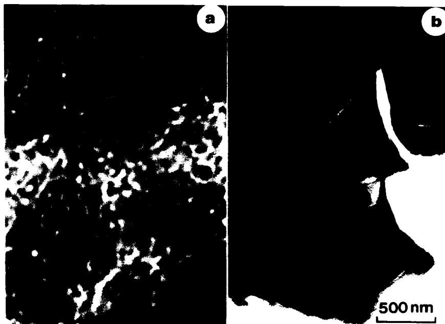
Fig. 3. Defocused FRESNEL micrographs showing the magnetic domain structure of a melt spun \text{Nd}_{4.5}\text{Fe}_{77}\text{B}_{18.5} -flake (a) and of a sintered Nd-(Fe,Co)-B:Ga magnet (b).
