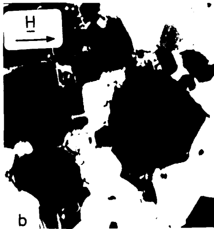
Fig. 13. Sequence of domain patterns in an aligned \text{Fe}_{77}\text{Nd}_{16}\text{B}_8 permanent magnet and varying magnetic fields. a) \mu_0 H_{\text{ext}} = 0 Tesla (thermally demagnetized state) b) \mu_0 H_{\text{ext}} = 1.4 Tesla (technically saturated state), c) \mu_0 H_{\text{ext}} = 0.4 Tesla (nucleation of reversed domains).
