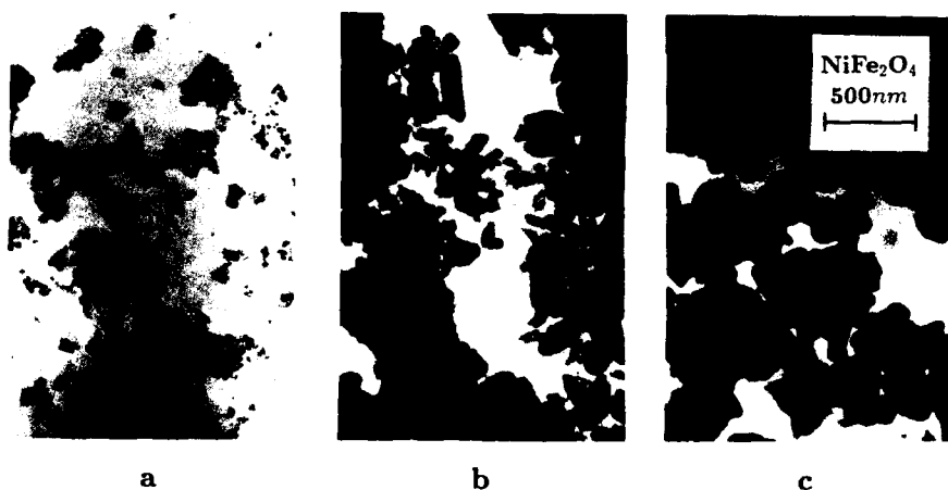
Fig. 1. Electron microphotographs of NiFe 2 O 4 nanometer particles prepared by chemical precipitation. Samples (a), (b) and (c) were made by altering the final thermal conditions.
