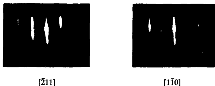
Figure 1 RHEED patterns from the two different azimuthal directions of the final Pd superlattice layer ( d_{Co}=4\text{\AA} , d_{Pd}=11\text{\AA} , N=30 ).
