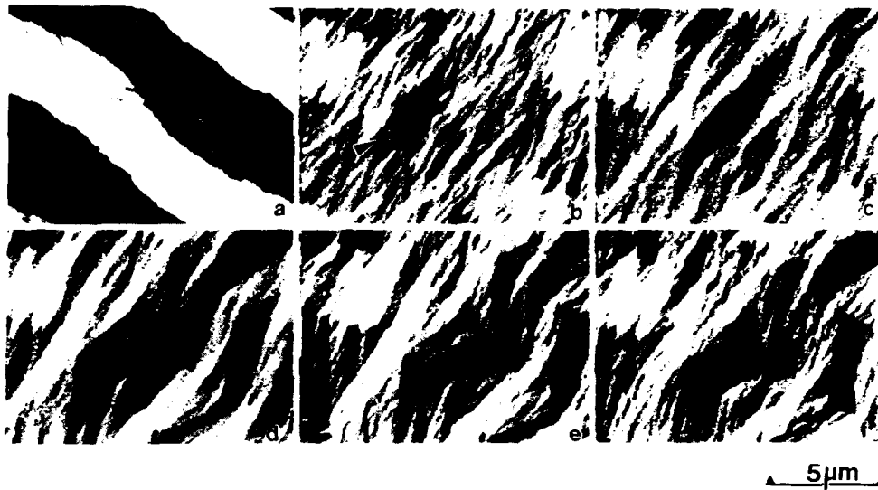
Figure 3. Domains in polycrystalline Co at a) & b) 20°C c) 200°C d) 270°C e) 400°C f) 20°C
