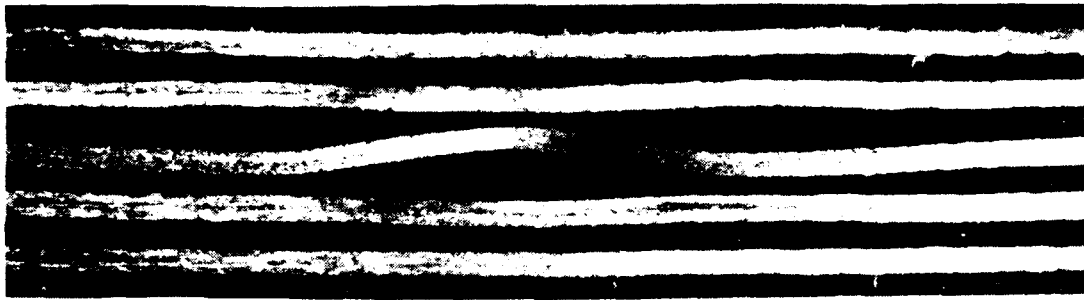
Figure 1. Moderate Layer Wave Geometry Fabricated in [90_2/0_2/90_2/0_2/90_2/0_2w]_s Laminate Using the Three Step Fabrication Method.
