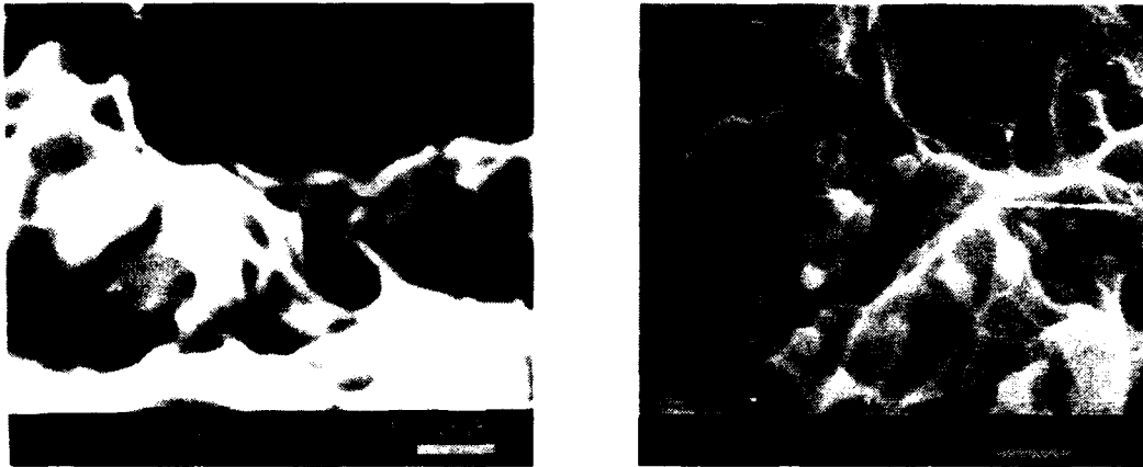
Figure 4. Scanning electron micrograph of fracture surface in a) \text{SiC}_p/\text{Al} and b) \text{SiC}_w/\text{Al} composites.
