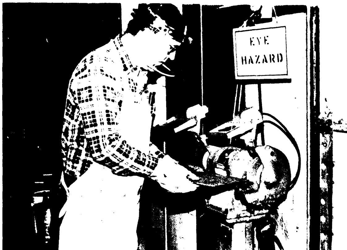
Figure IV-1. Spark testing metal on a grinding wheel.
