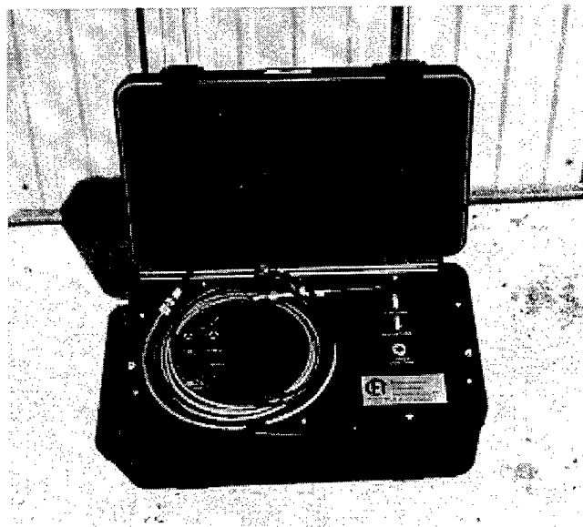
Figure 5. Down range unit receives signal from the walk around unit and retransmits signal to the command post
