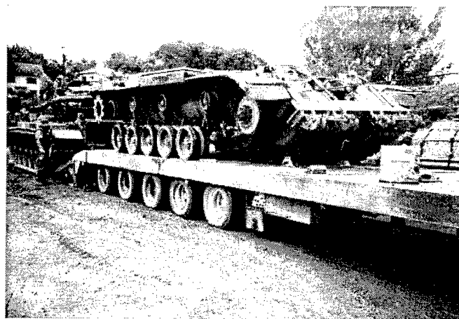
Fig. 9: After hitting an anti-tank mine, this panther sustained a damaged track and first road wheel. Here is the Panther on a transport vehicle awaiting repair.
