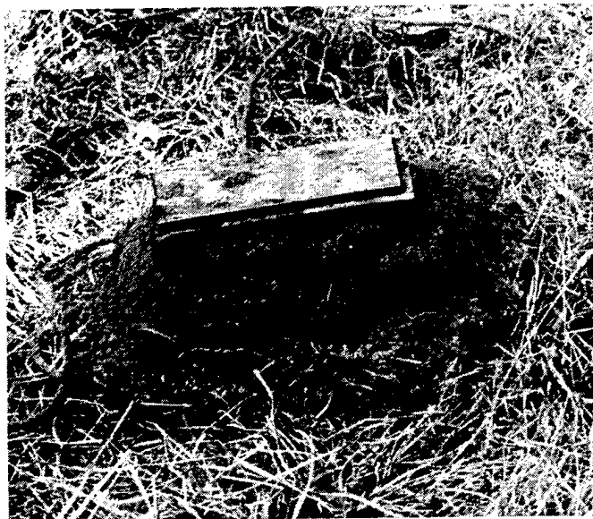
Fig. 5. Foam adhered well to some wooden box mines with wet and dirty surfaces.
