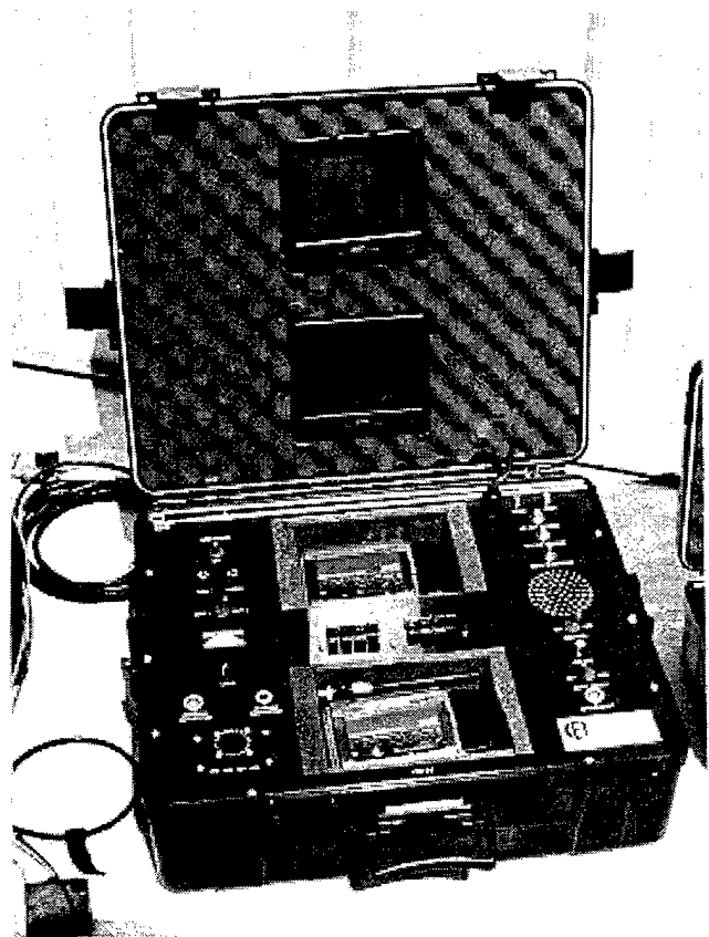
Figure 7. Command post unit is used to receive video from the minefield and transmit and receive audio to and from the deminer
