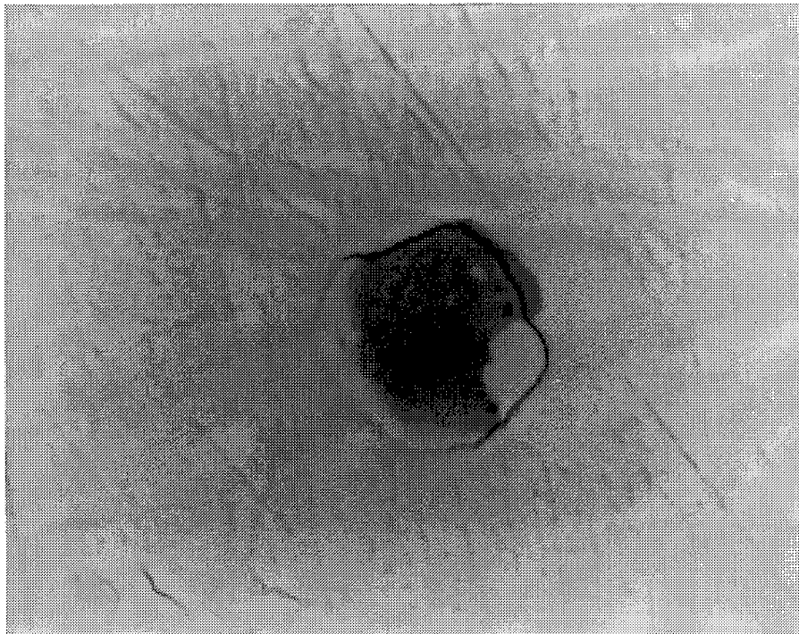
Photograph 20: Tray A-04, Silver/Teflon blanket showing mica protecting the Teflon surface from atomic oxygen and ultraviolet light degradation. 1100x magnification.
