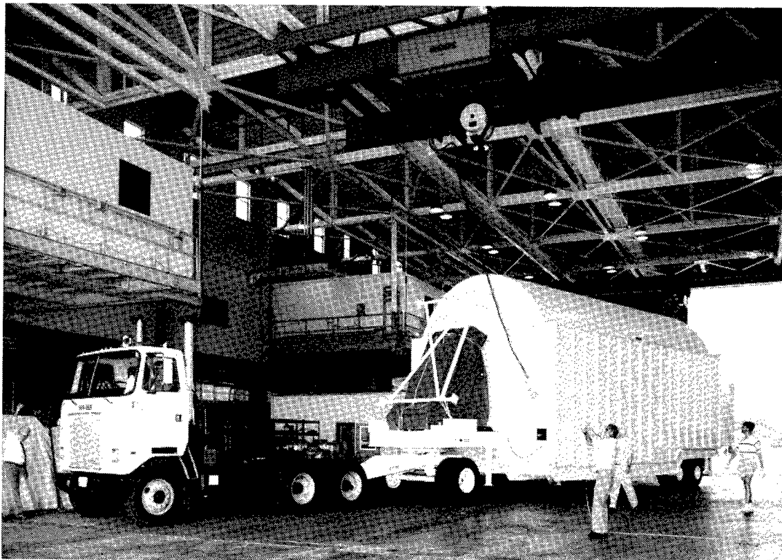
Figure 50.- LDEF Assembly and Transportation System (LATS) containing LDEF structure being placed in storage. (Photo KSC-390C-3976.11)
