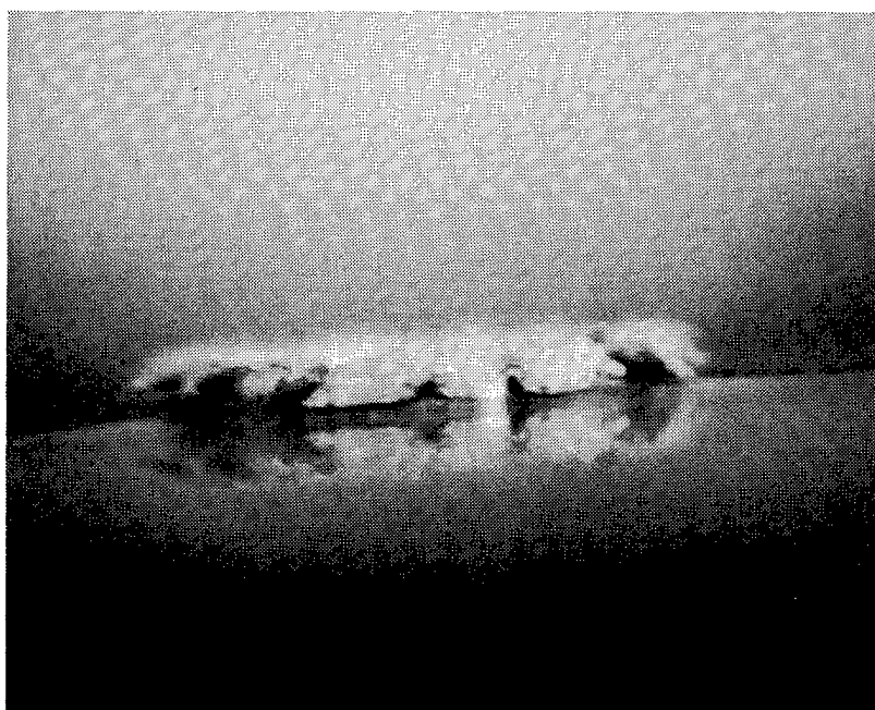
Fig. 4. Side view of a 2 mm diameter crater on plate F10H.
