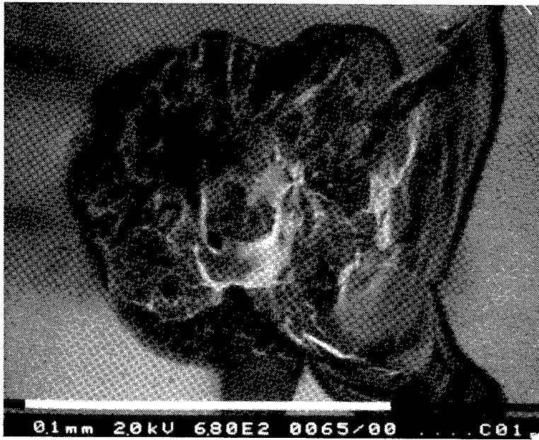
Figure 3. Small (top, No. 300-4) and large (bottom, No. 300-1) impacts on an IDE sensor . Note the four distinct morphological regions of the smaller feature: the central crater, the Al vaporization zone, the Al melt rim, and the area outside of the feature. An arrow points to a salt crystal identified in the SEM/EDS and is representative of one type of surface contamination. The larger impact feature has a spall zone that has obliterated ~1/2 of the Al vaporization zone and rim.
