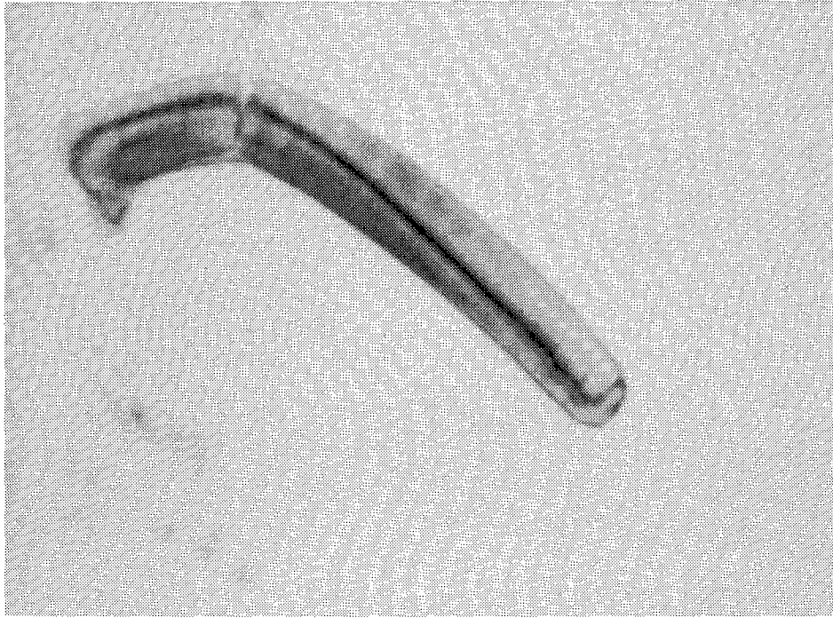
Photograph 9: Tapelift from the Shuttle Bay at Edwards showing ultraviolet modified nylon fiber. The photograph was taken using polarizing filters 15 degrees off crossed. 955x magnification.
