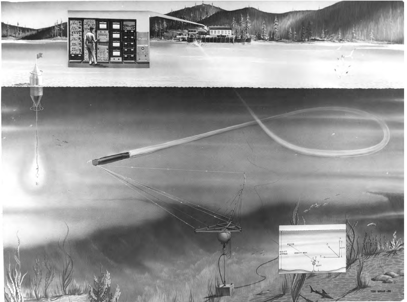
Three-Dimensional Range Installation in Hood Canal
