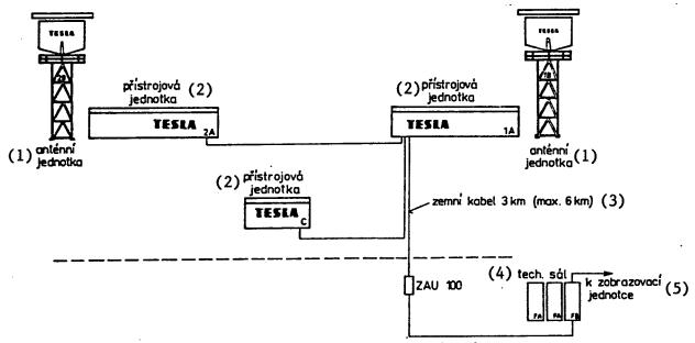
Figure 2. Composition of Model RL-61 Druzhba radar system.
