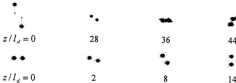
Fig.2. Sequential positions of solitons at different distances for soliton spiraling (the upper row) with cascaded nonlinearity ( \gamma A_1(0) = 15 , \theta = 0.3 , \Delta k l_d = 0.125 ) and (the lower row) phase-matching
