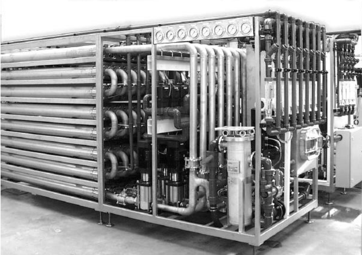
Fig. 3: low pressure reverse osmosis plant for grey water purification
