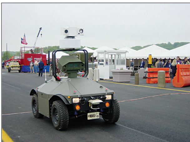
Fig. 4. The MDARS-Exterior SDD prototype in operation at the Force Protection Equipment Demonstration IV (FPED IV) at Marine Corps Air Station, Quantico, Virginia.
