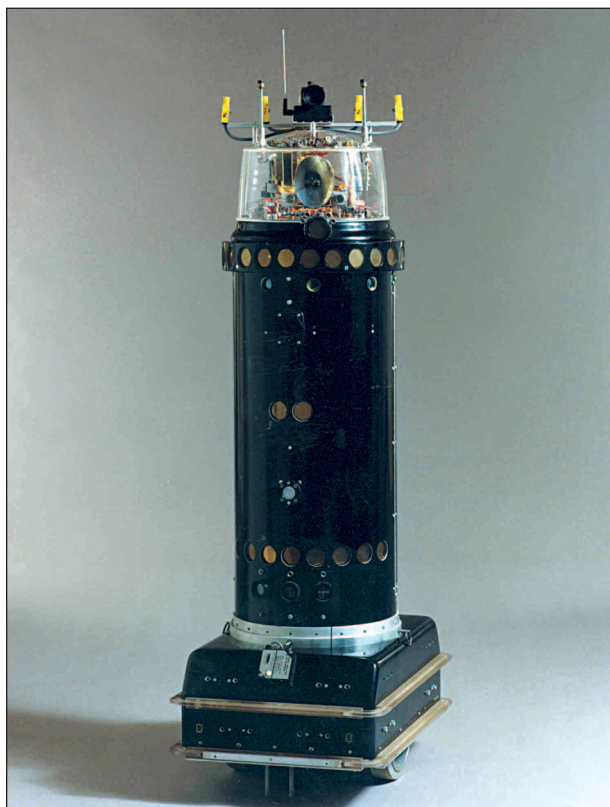
Fig. 1. ROBART II, a laboratory prototype used to develop the intelligent security assessment and autonomous navigation algorithms later employed on the MDARS-Interior security robot.
