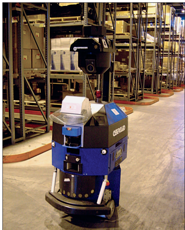
Fig. 3. The SDD version of the MDARS-Interior robot patrolling at Susquehanna Army Depot, Pennsylvania.
