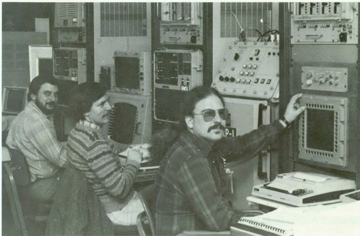
Gun Computing System—a major element of the AEGIS Destroyer Gun Weapon System—installed at NSWC Dahlgren for integration and certification testing.
