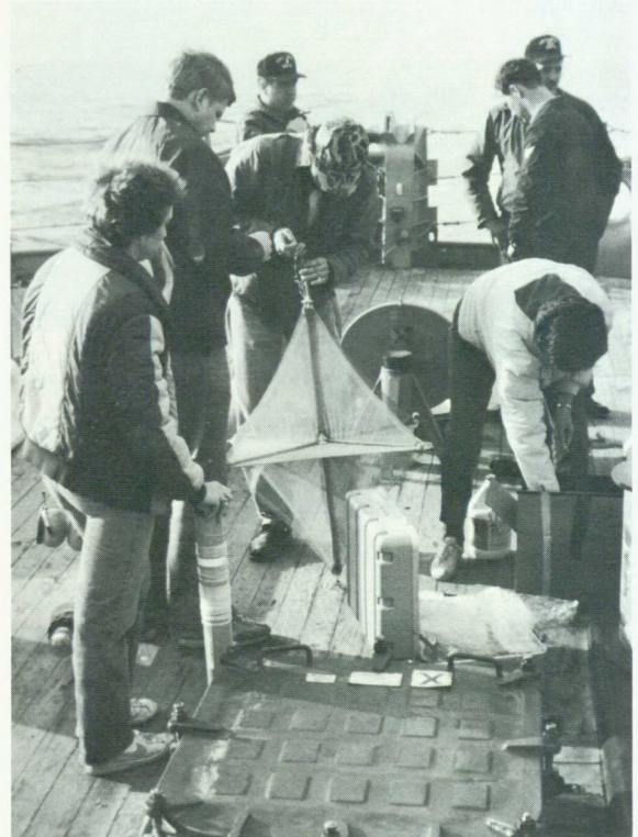
NSWC quick-response team aboard USS Iowa (BB-61) prepares corner reflector for the NSWC-developed surface target, designed to enhance gun operator efficiency.
