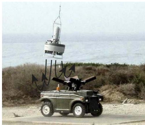
Figure 3. Ground Effect Illustration with Second Generation AUMS on MDARS
