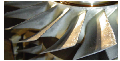
Stage I compressor blisk showing leading edge damage
