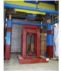
Test fixture to simulate dynamic loading of the arresting gear cable.
