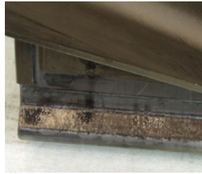
The coating is still intact on the dove tail section of a blade after completion of the ASMET.
