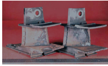
ASP1431 Stage I Vanes showing corrosion damage
