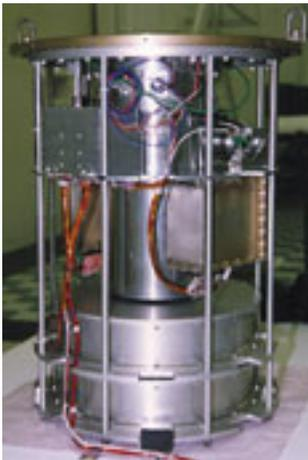
ARL Penn State is developing a thermoacoustic chiller (TRITON) with a 3-ton cooling capacity (10 kW) for shipboard application under ONR’s Environmental Requirements Advanced Technology (ERAT) Program. The cooling produced by the unit is created by a standing acoustic wave that expands and compresses inert gas within a porous plastic medium called a stack. Heat exchangers on each side of the stack carry away waste heat on one side and chilled water on the other side.
