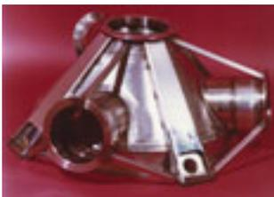
ARL Penn State has demonstrated the feasibility for affordable advanced laser cutting and welding techniques in concert with high-strength materials to produce welded transmission housings that will meet the performance requirements for ground combat vehicles, as well as rotorcraft and VSTOL aircraft employing high-performance transmissions. ARL is capable of establishing cost and performance benefits of a laser cut and welded housings versus conventional cast housings.
