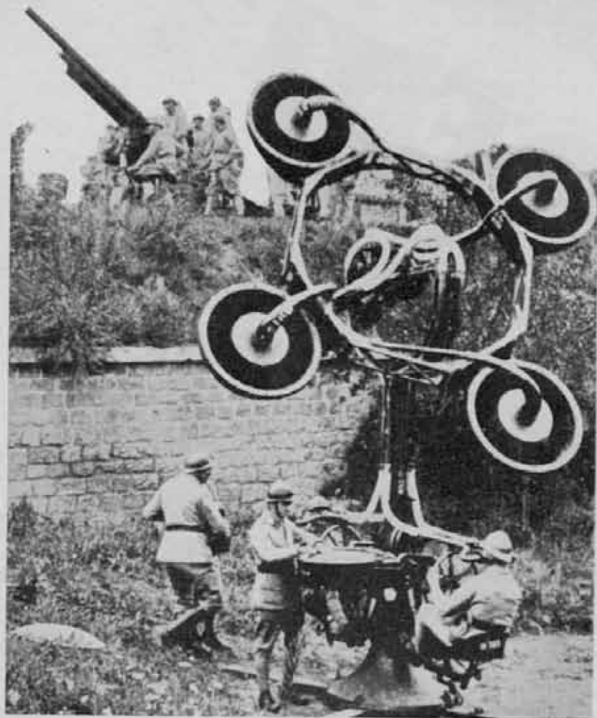
French sound locators and guns go into action near Paris. Especially worthy of note is the plotting device, which is an integral part of the sound locator.
