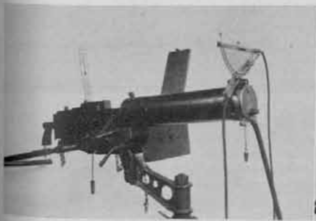
Figure 3 Sight attached to machine gun—front view.
