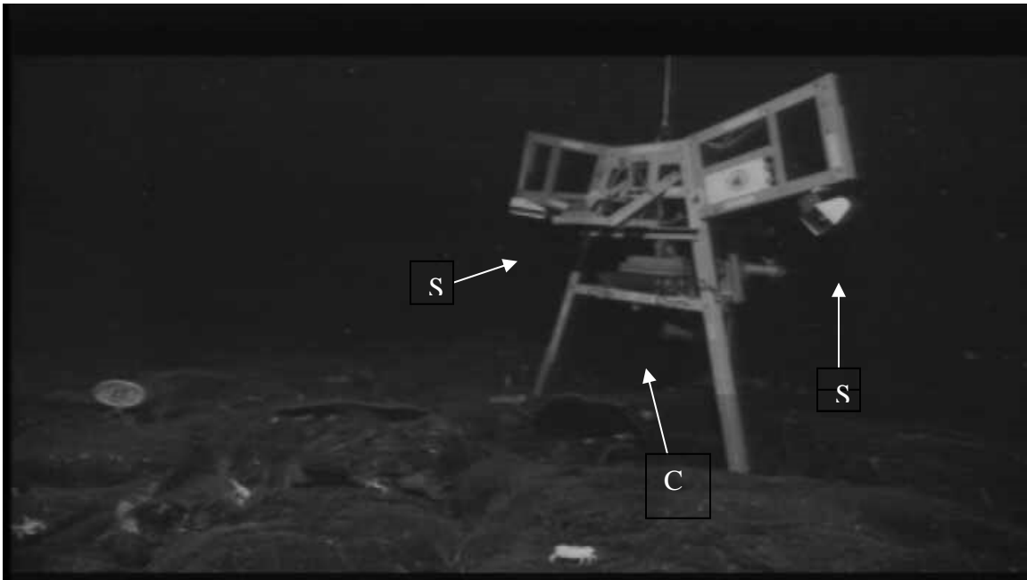
Figure 4.2 RatCam deployed on the seafloor over a fish hole. The strobes (S) and camera (C) are indicated by arrows.
