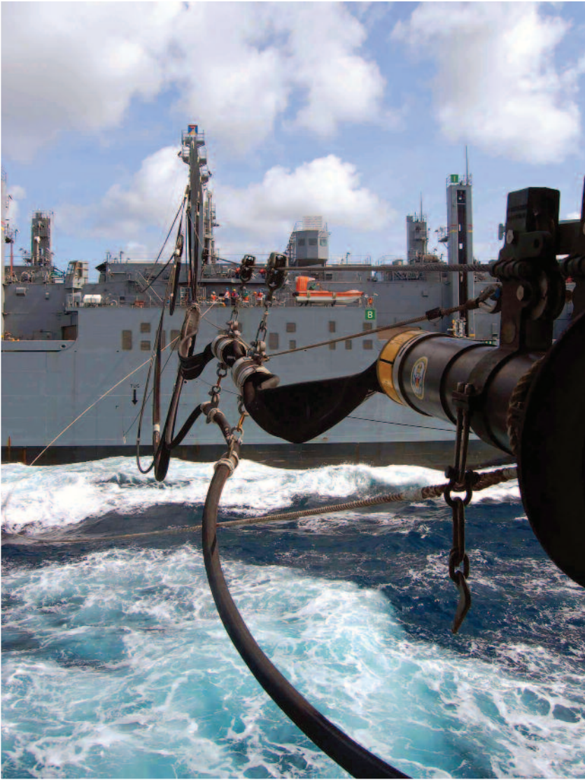
Fuel lines connect MSC hospital ship USNS Comfort and MSC dry cargo/ammunition ship USNS Robert E. Peary during Comfort's four-month humanitarian and civic assistance mission to Latin America and the Caribbean. Photo by A1C Ashley Garcia.
