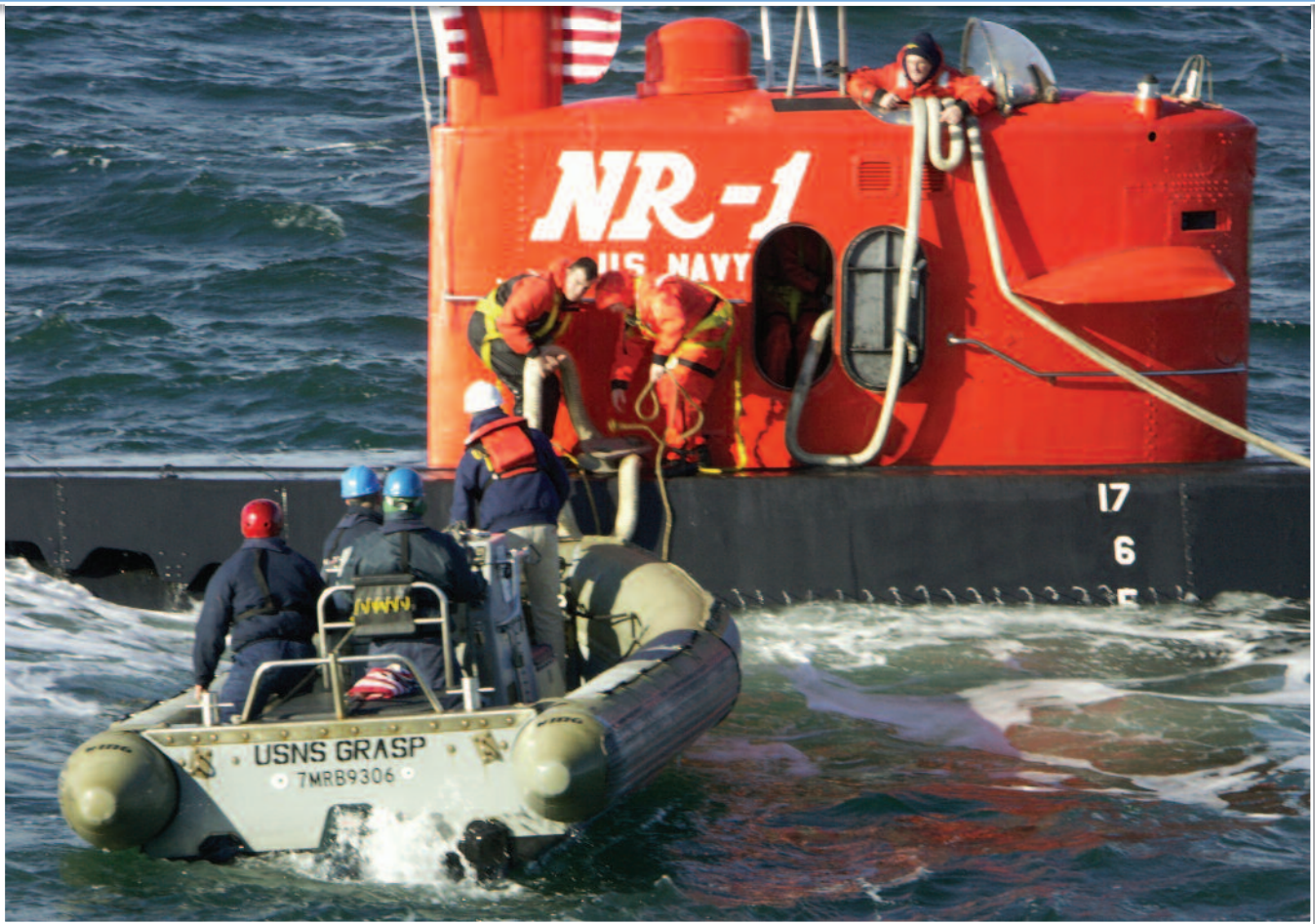
MSC rescue and salvage ship USNS Grasp mariners assist the crew of the U.S. Navy's deep-submergence submarine NR-1 with the towline hookup in Groton, Conn., in December 2008. Photo by Bill Cook.
