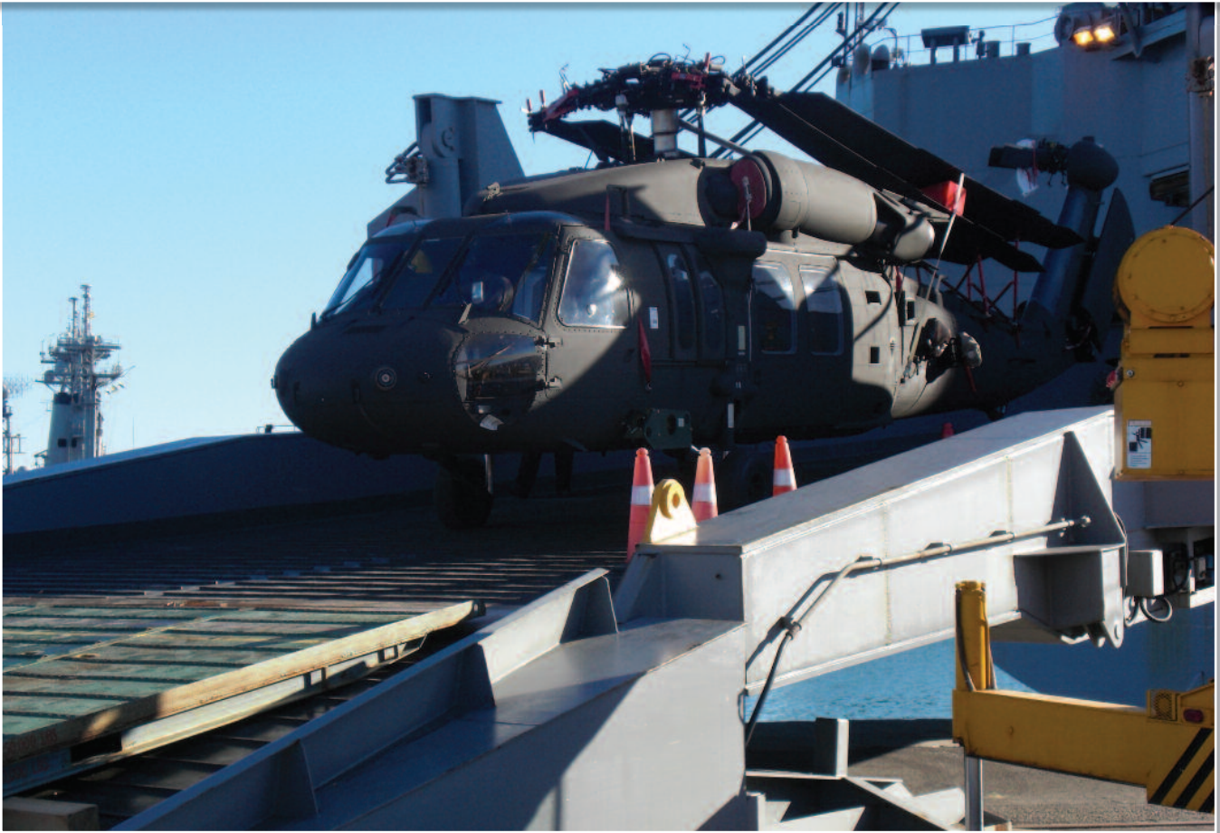
A helicopter is discharged via the stern ramp of MSC large, medium-speed, roll-on/roll-off ship USNS Benavidez in Rota, Spain, in November 2008. Photo by Robert Foster.
