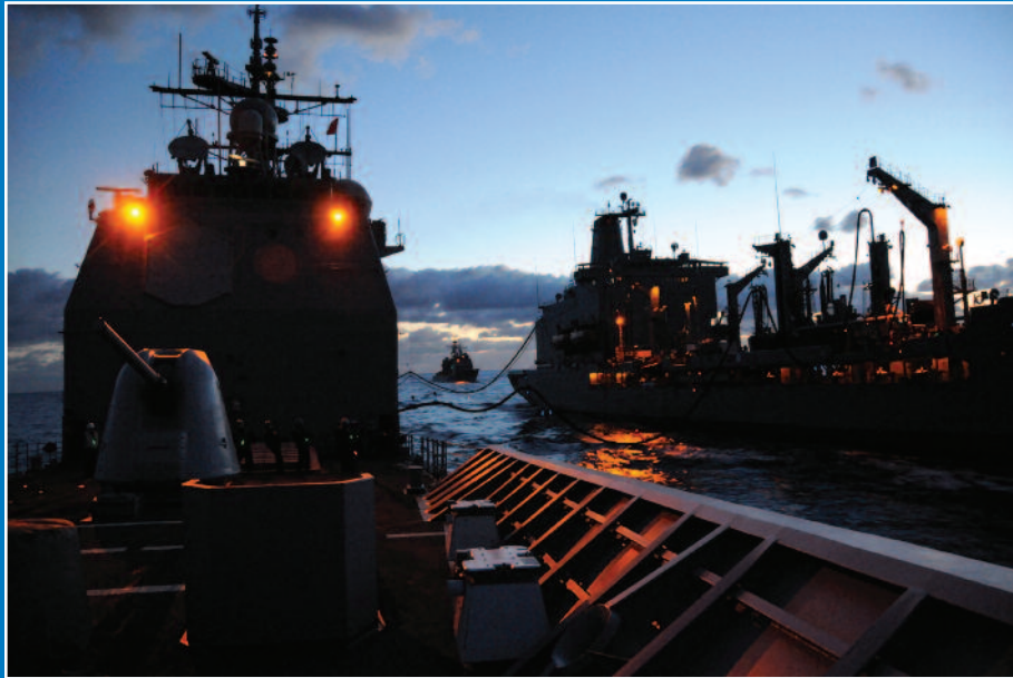
MSC fleet replenishment oiler USNS Big Horn conducts an underway replenishment with guided-missile cruiser USS Vicksburg in the Atlantic Ocean. Photo by Ensign Marc D. Schron.
