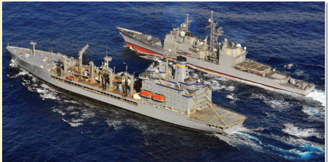
MSC fleet replenishment oiler USNS John Ericsson stands by as guided-missile cruiser USS Lake Champlain, right, approaches for a replenishment at sea in the Western Pacific Ocean. Photo by MC2 Daniel Barker.
