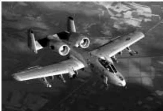
The A-10 Thunderbolt II has a Night Vision Imaging System (NVIS), a goggle-compatible single-seat cockpit forward of its wings, and a large bubble canopy that provides the pilot all-around vision. Titanium armor protects both the pilot and parts of the flight-control system.
