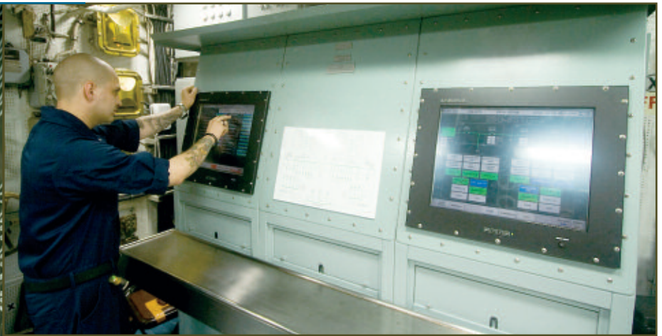
Above: The Sailors' electric plant situational awareness was very limited with the analog electric plant controls providing basic SSTG only information prior to installation of PMP.
