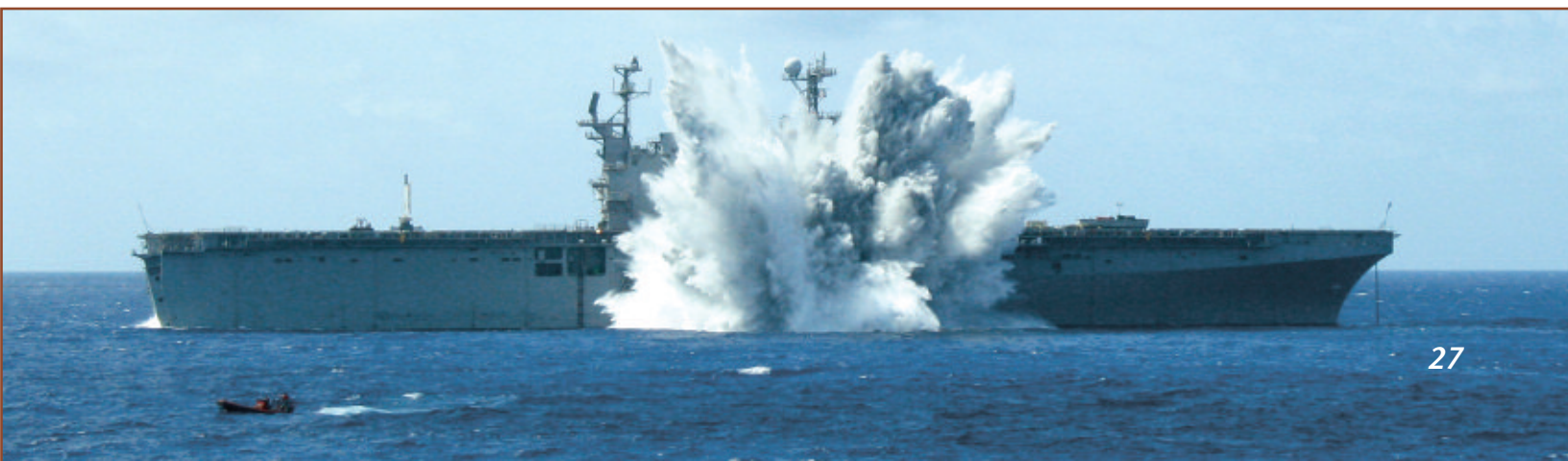
Below: Shock test of Ex-USS Saipan plume shot.
