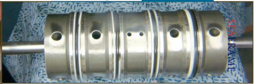
Above: Slide and sleeve assembly—the internal moving components of the valve.
