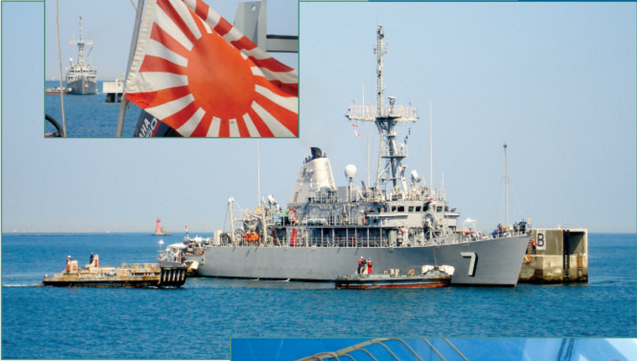
Above: USS Patriot (MCM 7), an Avenger Class mine countermeasures ship, is pushed into place at the deperming station in Yokosuka harbor.
