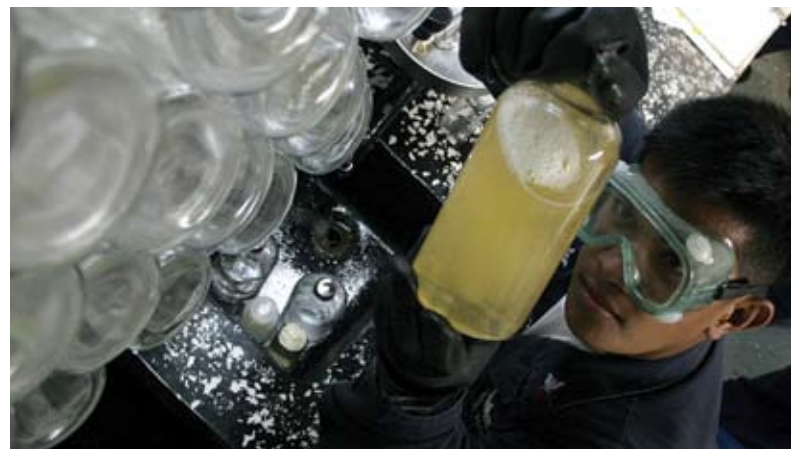
A gas turbine system technician takes a fuel sample aboard the guided-missile destroyer USS Stethem (DDG 63). (U.S. Navy photo by Ensign Danny Ewing Jr.)
