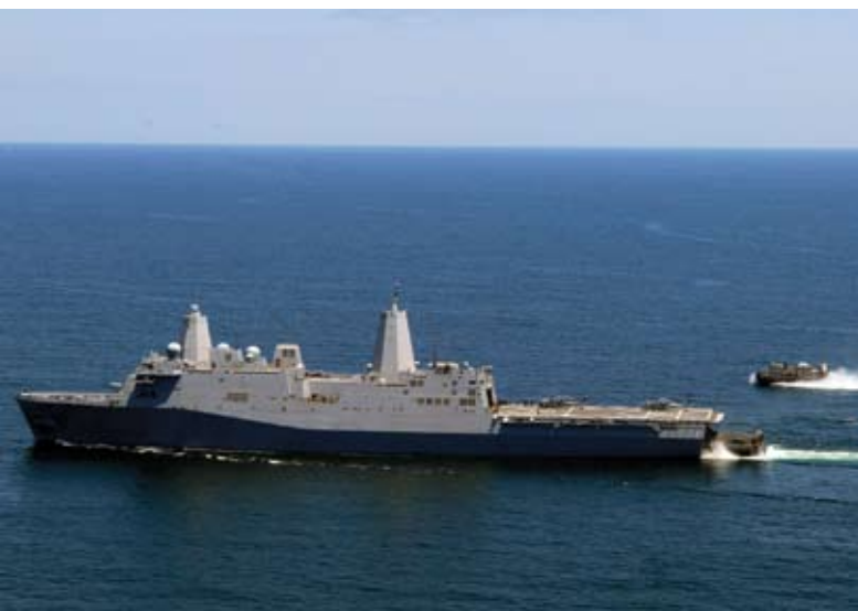
Landing craft air-cushioned vehicles disembark from the well deck of the amphibious transport dock ship USS Mesa Verde (LPD 19) for an amphibious landing demonstration near Mayport, Fla. (U.S. Navy photo by Mass Communication Specialist Seaman Patrick Grieco)
