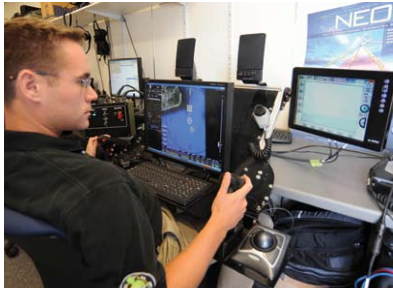
Sean McCready, NSWC Dahlgren software engineer, remotely controls the Navy Expeditionary Overwatch (NEO) unmanned surface vehicle sensor suite during a demonstration. (Photo courtesy of Northrop Grumman Corporation)
