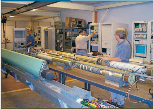
The Communications and Control Lab is used to certify, modify, and repair submarine antennas and related components. Photo provided by James Stiles, NSWC Carderock Division.
