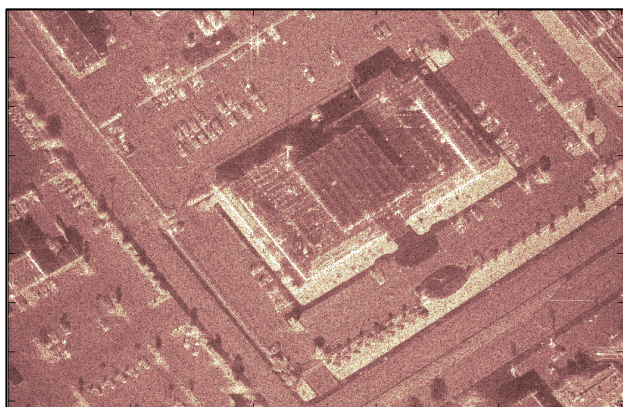
Figure 3. SAR image from a Sandia National Laboratories (SNL) Ku-band Mini-SAR. Image courtesy SNL from http://www.sandia.gov/RADAR/sar-data.html .
