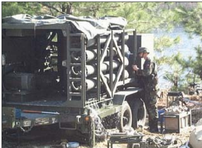
Figure 3. Army 600-gph trailer-mounted ROWPU.
