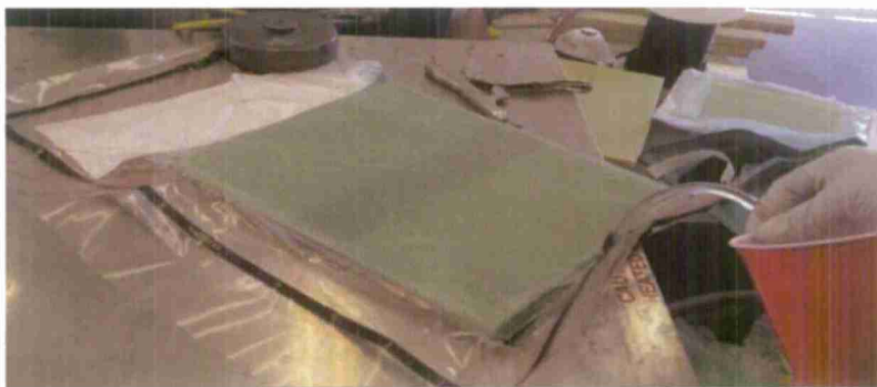
Figure 36 - VaRTM composite lay-ups resin flow
