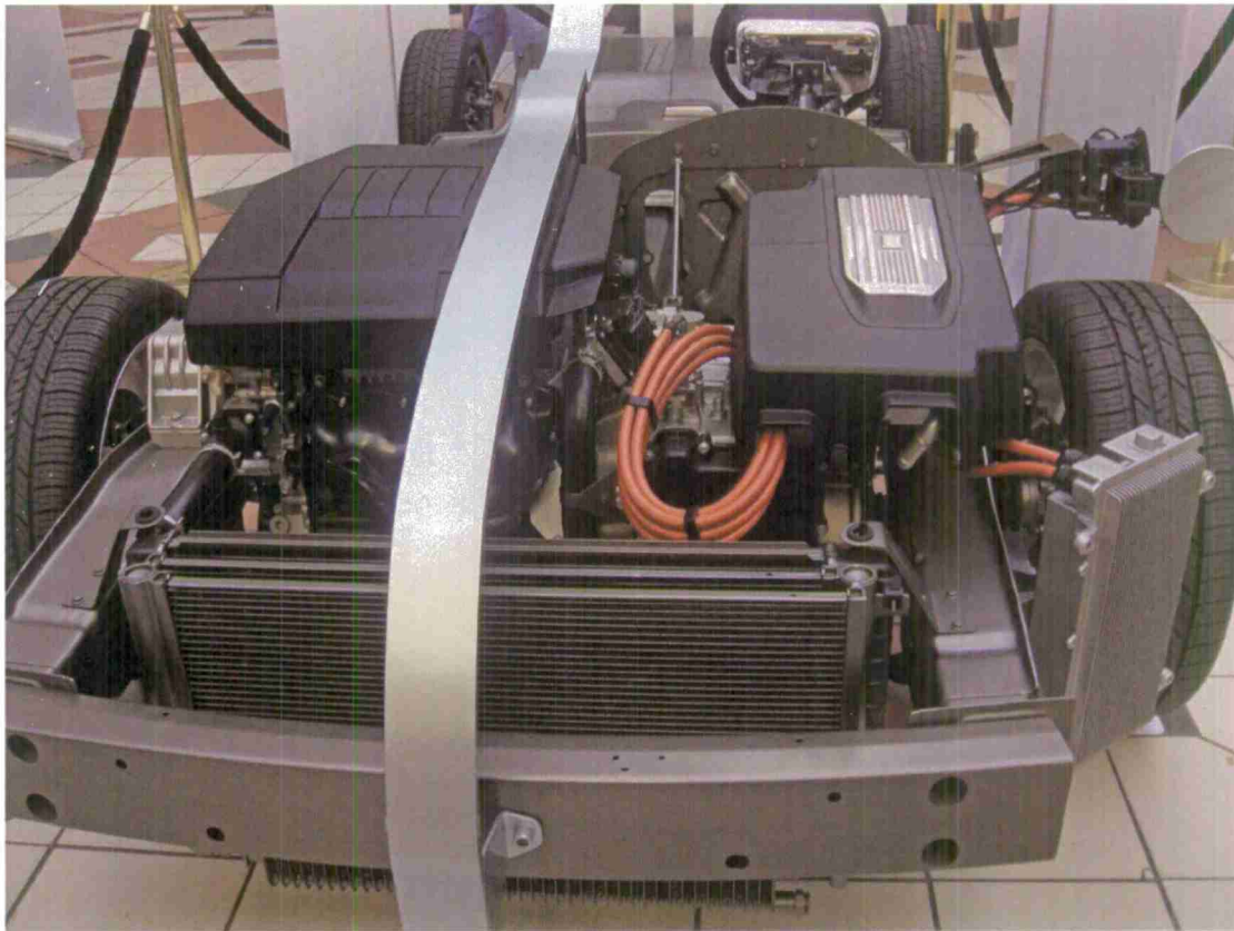
Fig. 1. Engine compartment of Chevy Volt showing conventional combustion engine on left side and the electric motor and power electronics on the right side. (photo from http://en.wikipedia.org/wiki/File:Chevy_Volt_DCA_01_2010_8811.JPG )
