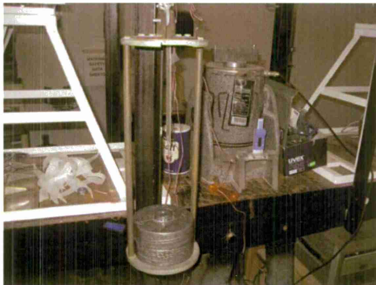
Figure 118 - Applied loading for material calibration
