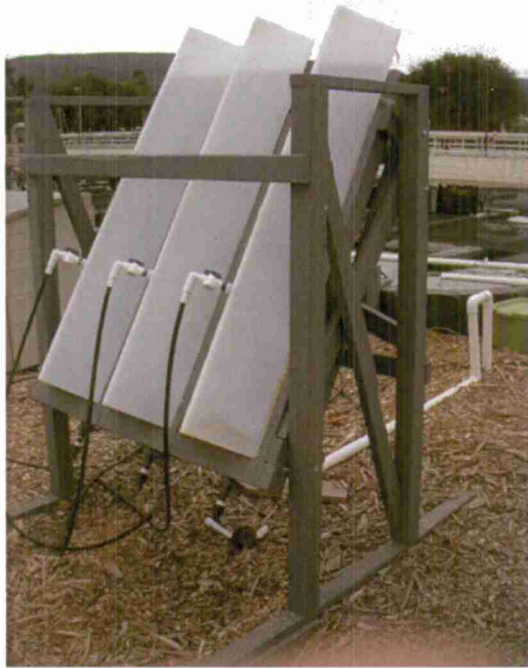
Figure 3: Cal Poly Algae Field Station Tube Settlers for algae-water separation.
