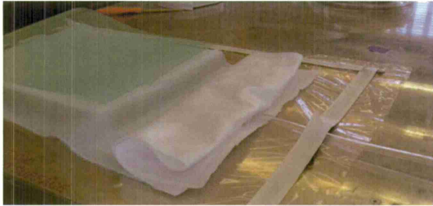
Figure 33 - Stacked VaRTM lay-up before vacuum bagging
