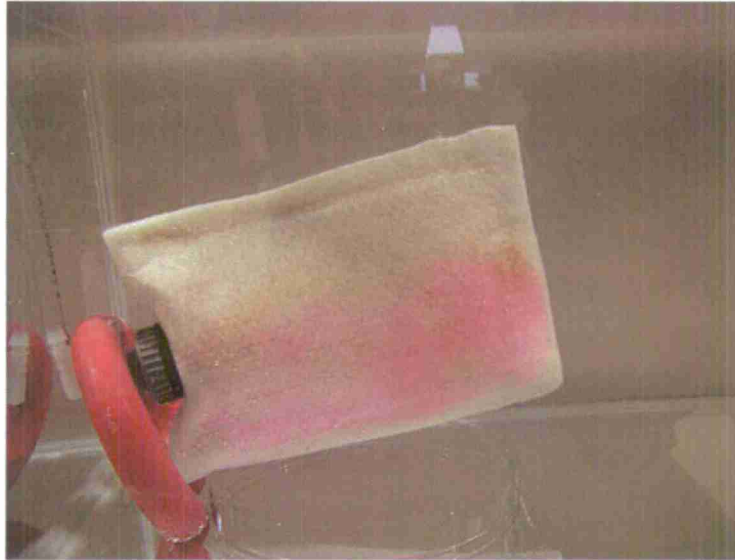
Figure 10: A dirty, previously used rectangular filter with a middle bulkhead fitting used in experiment D-2. Scale: the large diameter bulkhead fitting on the left side of the filter measures 3.65 cm in diameter.
