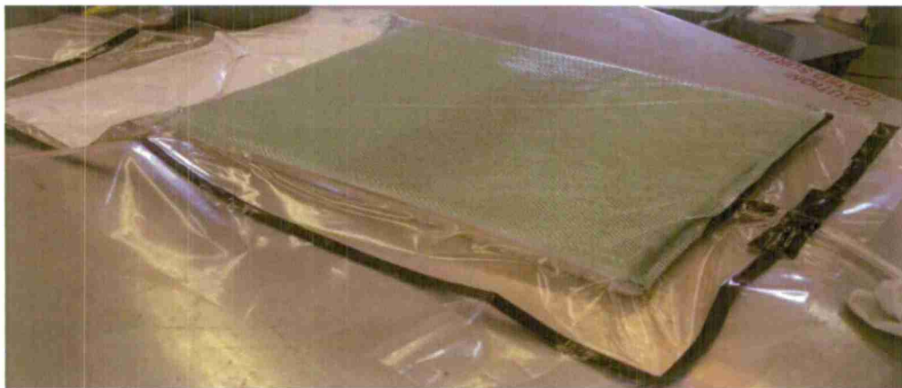
Figure 34 - Vacuum bagged composite sandwich structure after lay-up
