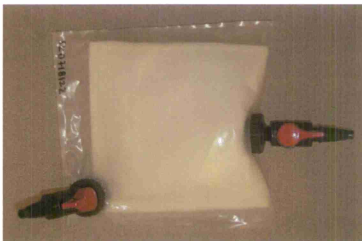
Figure 4: 2-ply nom.-abs. filter tested in experiment H-3. Scale: the large diameter bulkhead fitting measures 3.65 cm in diameter.
