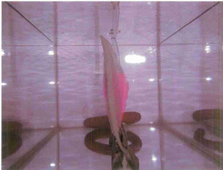
Figure 11: Thin plume of rhodamine dye and water mixture observed along clean, rectangular filter tested in experiment D-2. Scale: the clear tubing in the upper half of the picture measures 0.75 cm in diameter.
