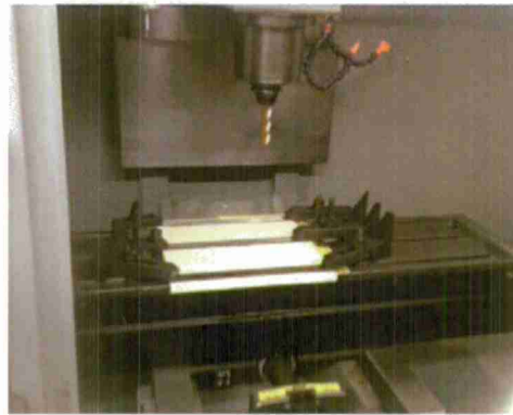
Figure 41 - Milling of foam for DADs
