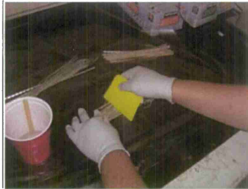
Figure 5 - "Wet Layup" Technique
