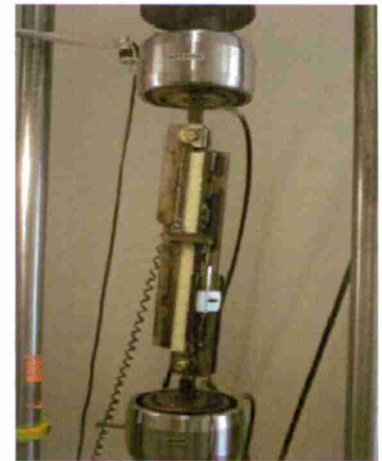
Figure 15 - Composite sandwich structures under shear testing (ASTM C273)
