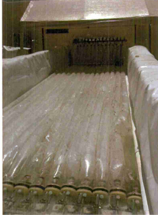
Figure 3. Photograph of the heat transfer pond designed and built by Extreme Exchangers senior project team in Bonderson Yard.
