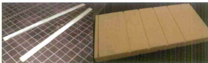
Figure 13 - Shear key rods and grooves milled into foam core
