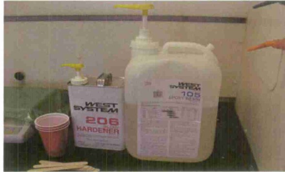
Figure 35 - West System resin and hardener used for lay-up
