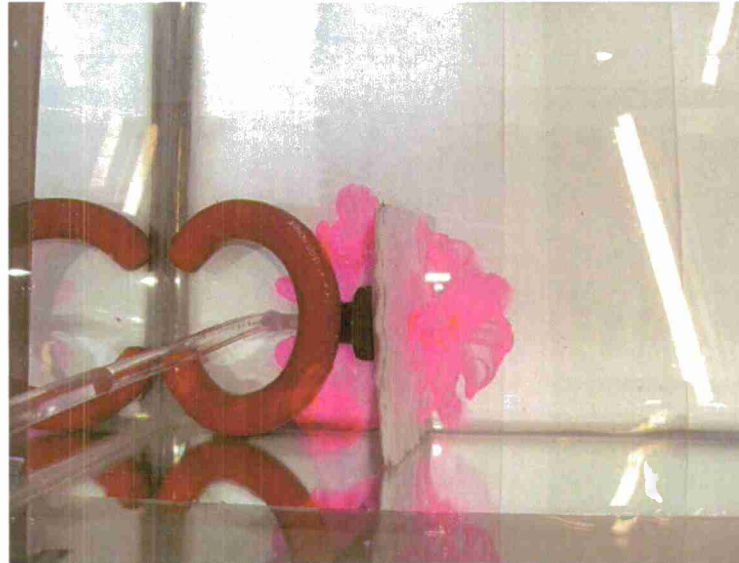
Figure 8: Plume of rhodamine dye and water mixture jetting out of the internal chamber of a square filter in experiment D-1. Scale: the large diameter bulkhead on the left side of the filter measures 3.65 cm in diameter.
