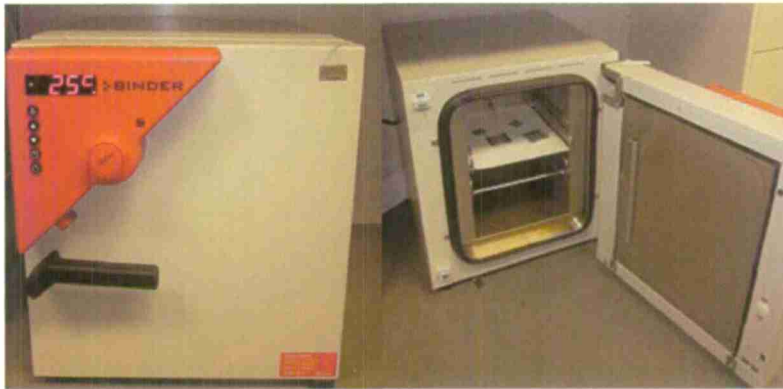
Figure 4. Programmable oven to melt wax patterns into Nitrocellulose membranes.
