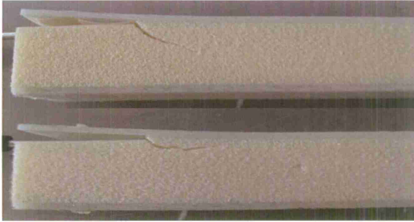
Figure 61 - Monotonic failure of test specimens with 1.0 inch initial delamination
