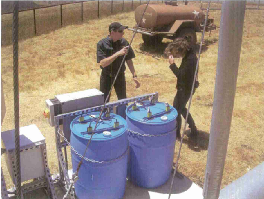
Figure 4: Resistive load bank for the wind turbine. The two barrels are filled with water and absorb heat from eight resistance coils. The trailer in the distance holds extra water with which the barrels are refilled periodically. The effect of the favorable wind resource at the wind turbine site is visible in the reaction of one of the onlookers.
