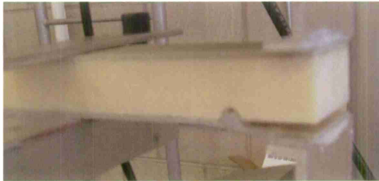
Figure 62 - Monotonic failure shear key delamination
