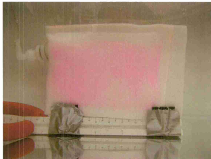
Figure 9: A clean, rectangular filter with a high bulkhead fitting used in experiment D-2. Scale: the rectangular filter measures 10.2 cm by 15.2 cm.
