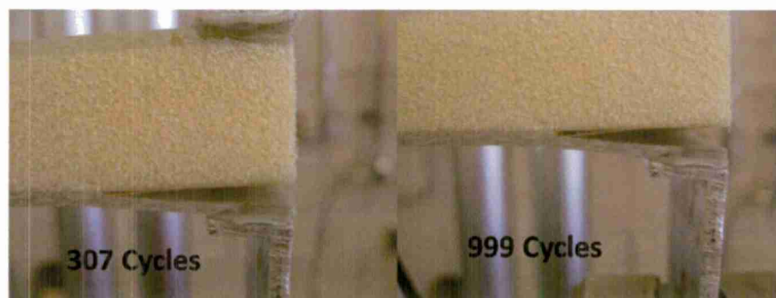
Figure 68 - 1.0 inch delamination fatigue crack propagation through foam
