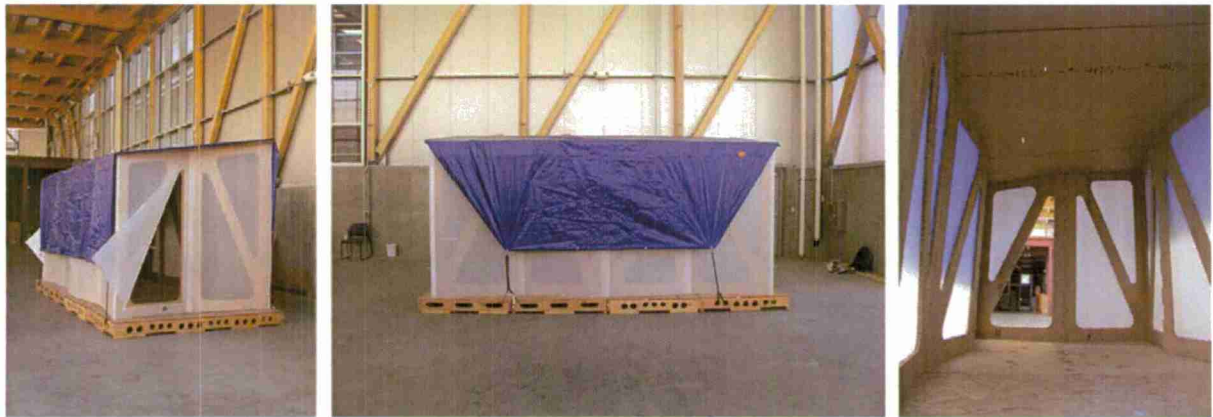
Figure 3: Prototype 4, the results of our work in Phase 2. Simplification of the roof plus the use of cardboard resulted in a lighter structure with connections that led to the use of zip ties.
