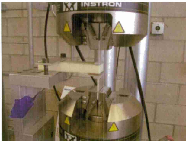
Figure 45 - 100 kN load cell Instron grip configuration
