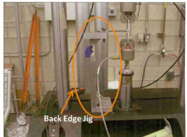
Figure 46 - 1 kN load cell configuration and back edge jig
