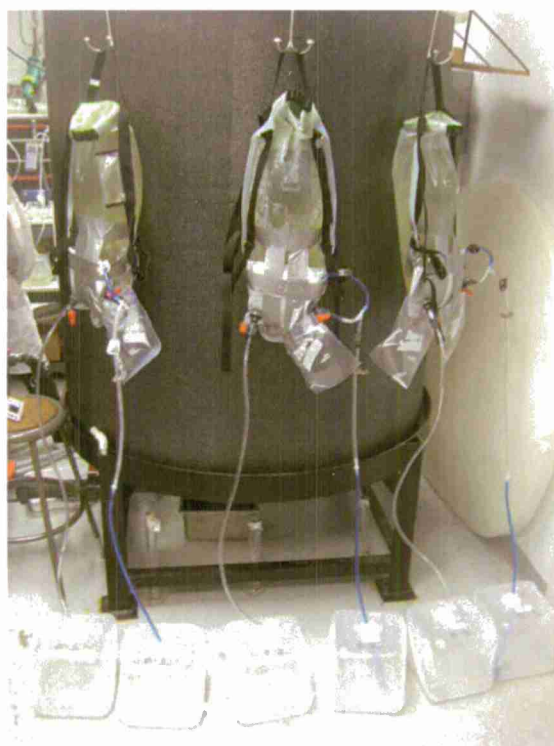
Figure 6: Testing in triplicate at BioVir Laboratories. Seale: the tubing measures 0.75 cm in diameter. The sandwich bags hanging below the waterbags were taped in place to catch any leaks from an imperfect prototype fitting.
