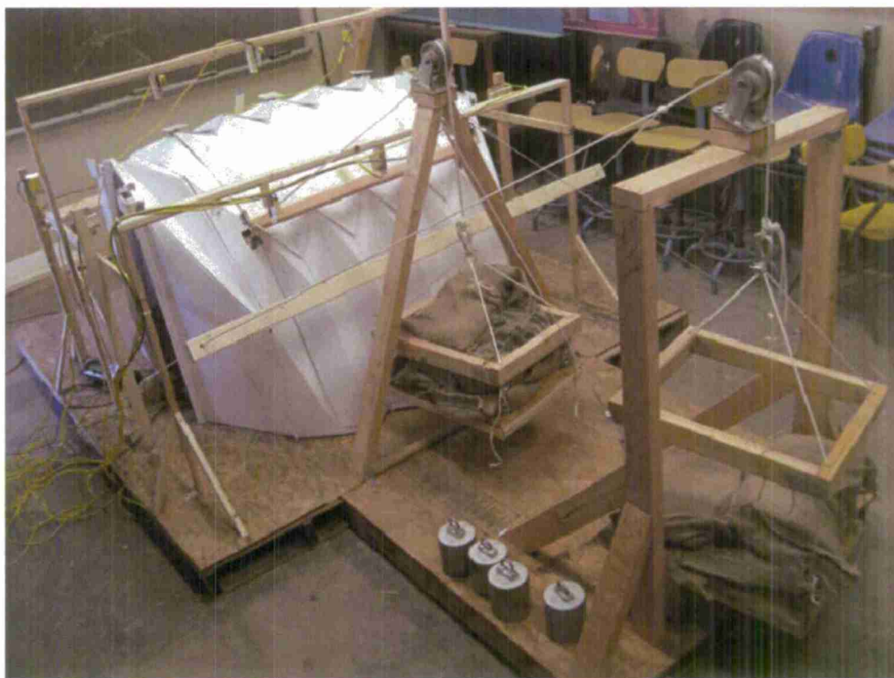
Figure 1. Half-Scale Origami Disaster Shelter Mock-Up, Simulated Wind Load Testing Set-Up (Ref. 19, page 142).
