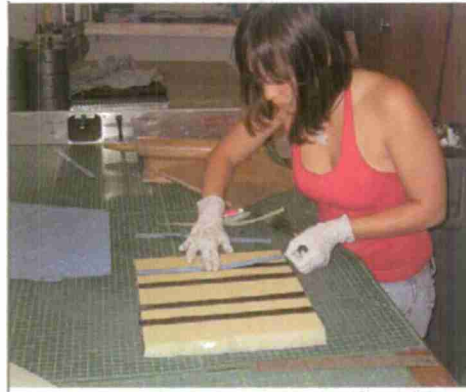
Figure 43 - DADs being inserted into foam slots
