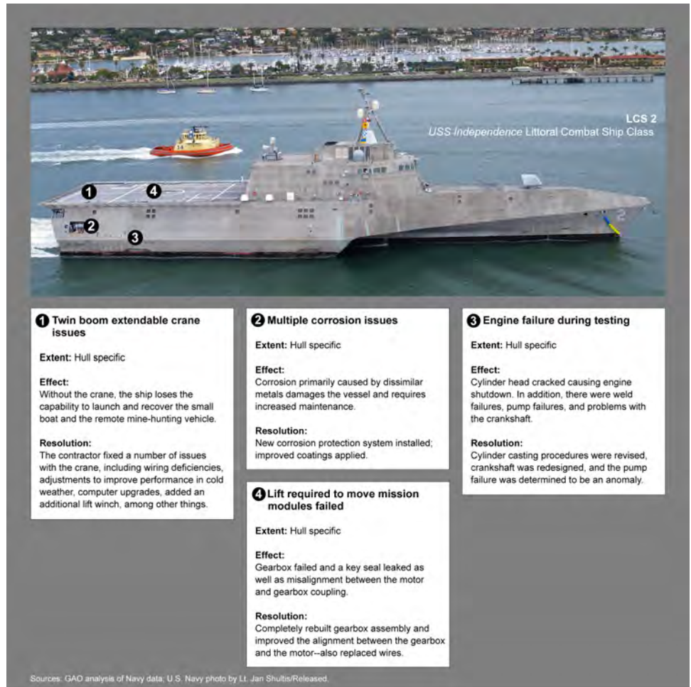
Figure 19: Selected Quality Issues on USS Independence (LCS 2)
