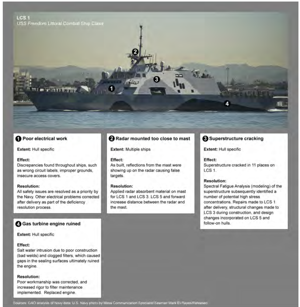
Figure 18: Selected Quality Issues on USS Freedom (LCS 1)
