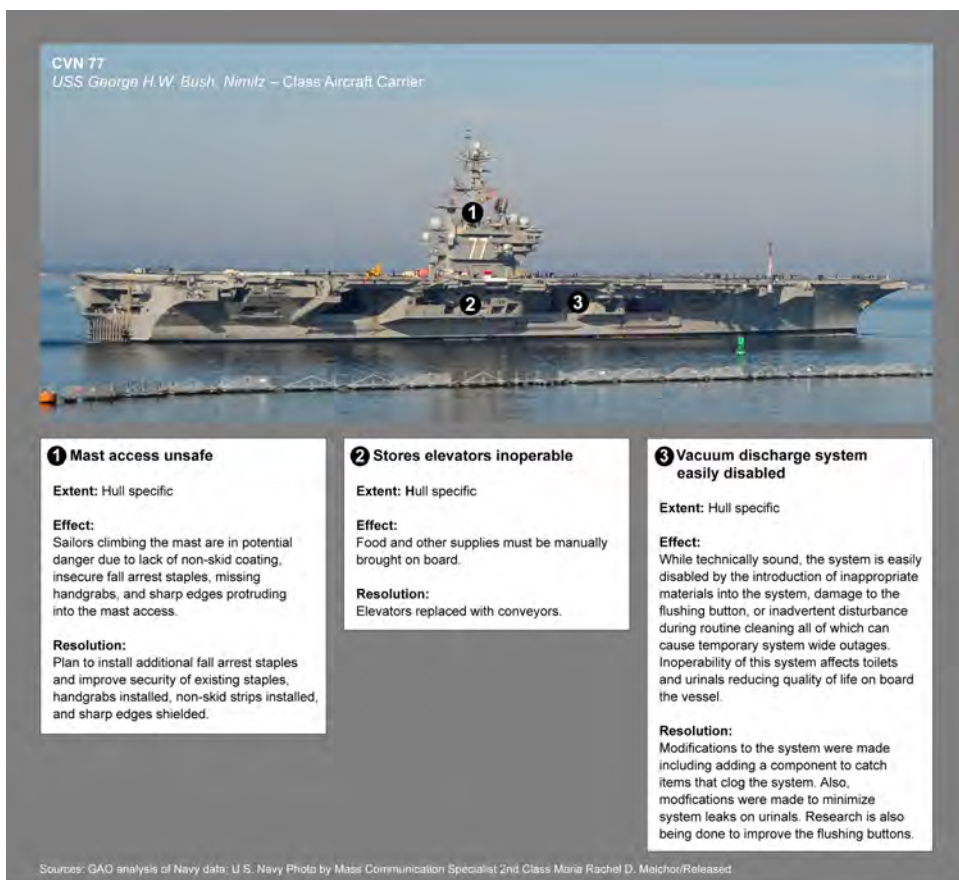
Figure 16: Selected Quality Issues on USS George H.W. Bush (CVN 77)
