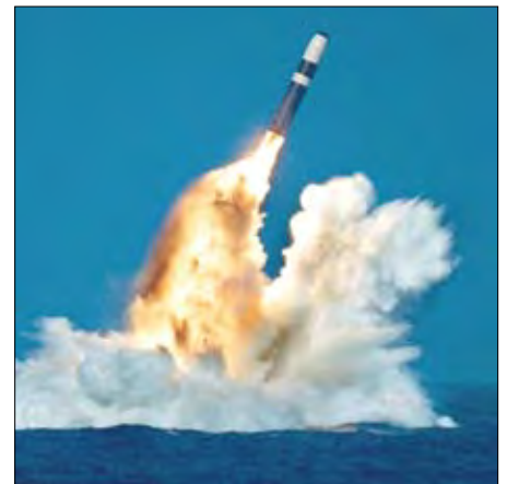
The Trident missile, named after the trident, is an intercontinental ballistic missile (ICBM) which is armed with nuclear warheads and is launched from submarines (SSBNs), making it a SLBM.
