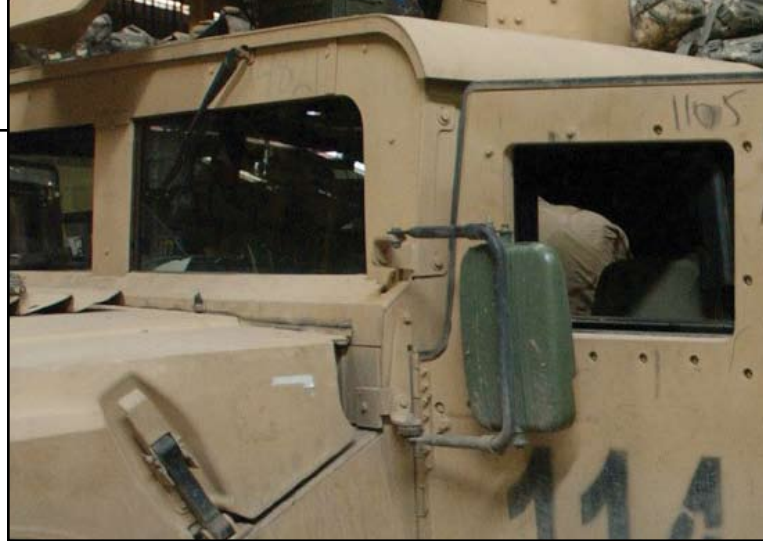
A welder with the 503d Maintenance Company disassembles an old combat lock on a humvee door at Forward Operating Base Falcon. He will replace it with a new combat lock with a single-action mechanism that allows the door to be opened with one motion.
