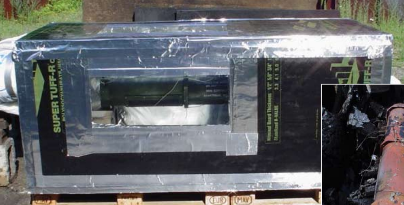
Above, a MACS container is positioned for a slow cookoff test. At right, the container is shown after a successful test in which the munition did not explode.
