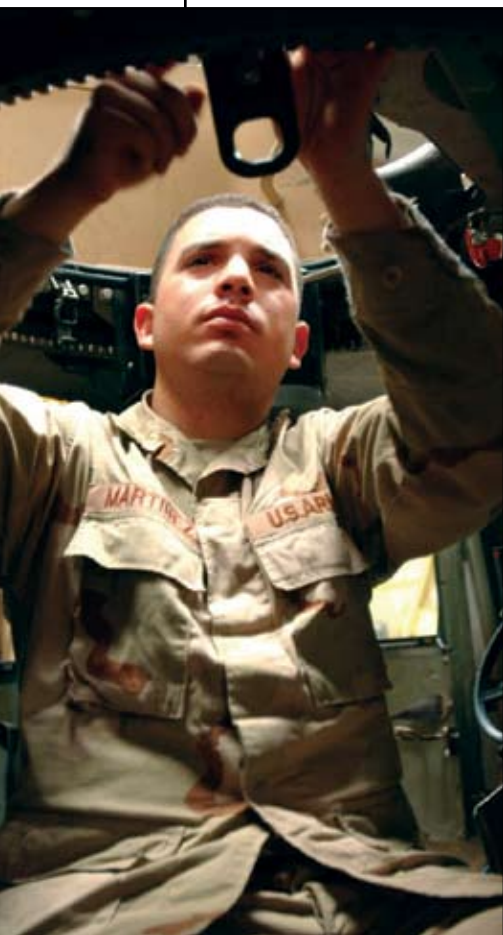
A Soldier installs a gunner's harness bracket on a humvee. This gunner restraint keeps the Soldier from being ejected during a rollover or sudden stop.
