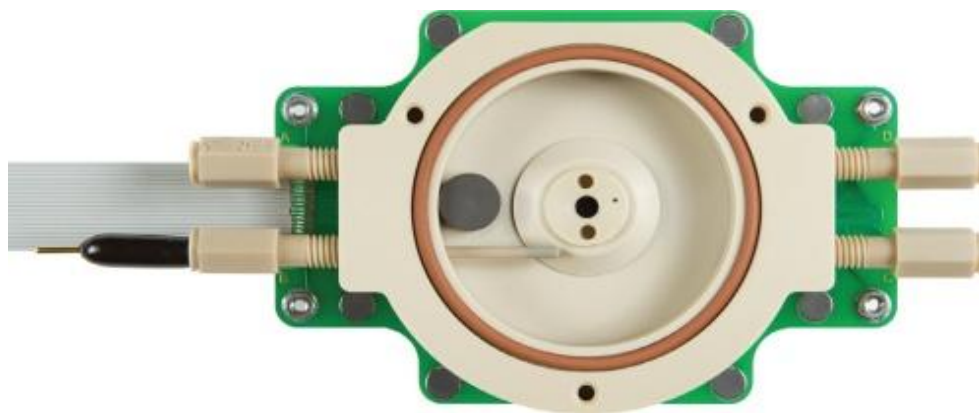
Figure 2. Electrochemical cell for in situ AFM measurements.
