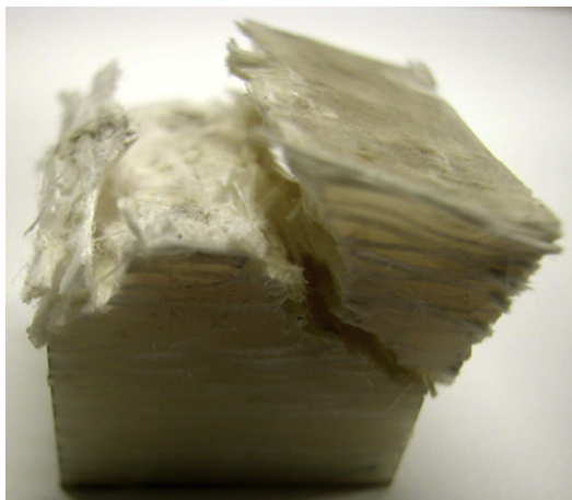
Fig. 8. Typical damage surface of a fractured specimen.
