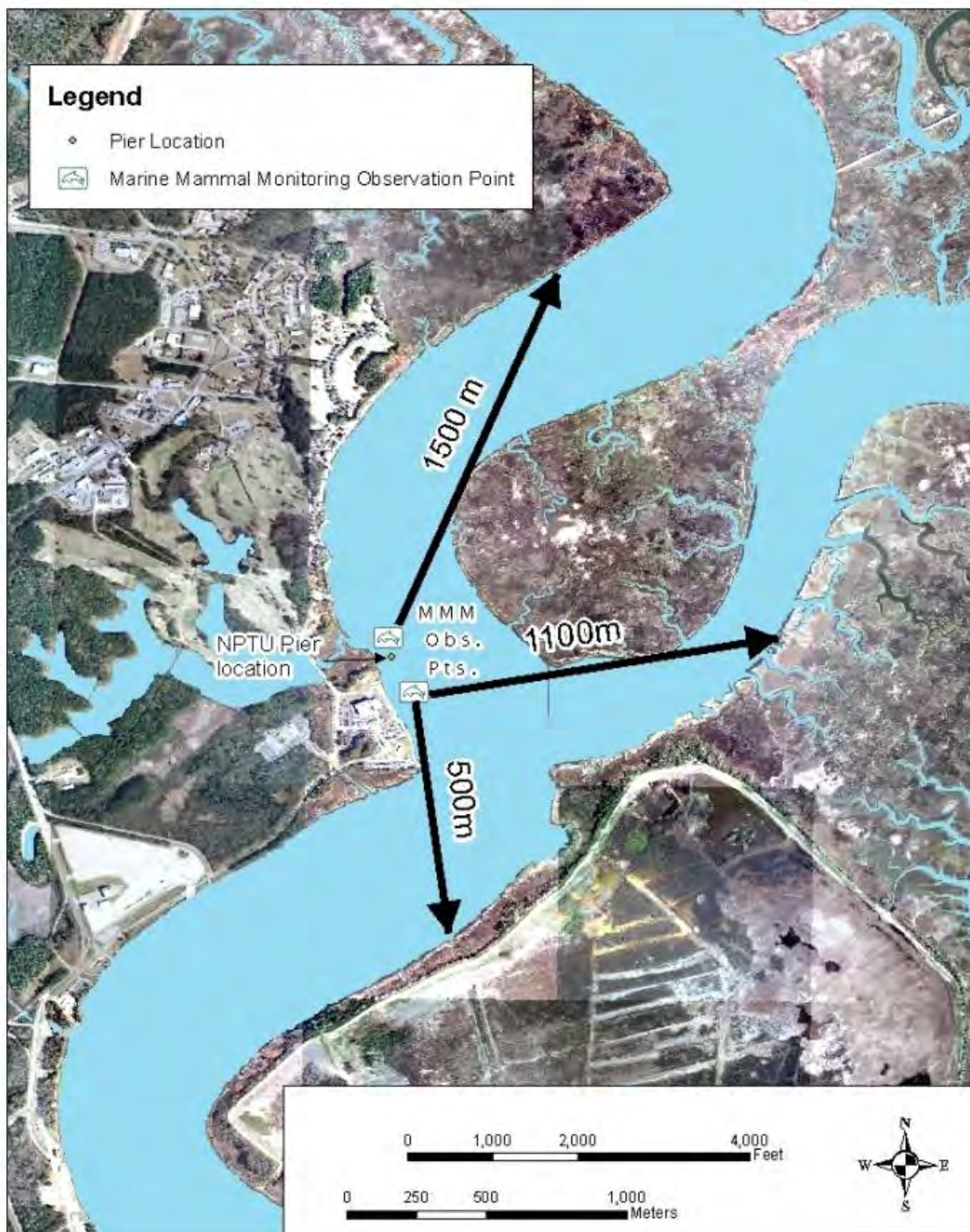
Figure 1. Lines of sight for marine mammal observes employed during steel pile driving at the Navy Nuclear Propulsion Test Unit, Charleston, South Carolina. Observer points are approximate. Lines of sight show the maximum distance sound can travel to each shoreline.
