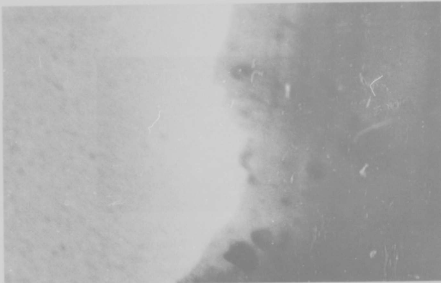
Fig. 87a Bright Field Image of Edge of Particle of Ground \beta -Rhombohedral Boron, Showing Faint Parallel Striations. 31,500 \times , P923
