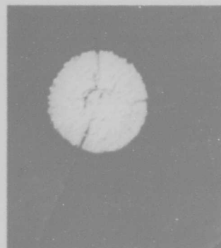
Fig. 21 Core Structures in Boron Filaments Deposited Under Different Conditions. (Astro Material A
