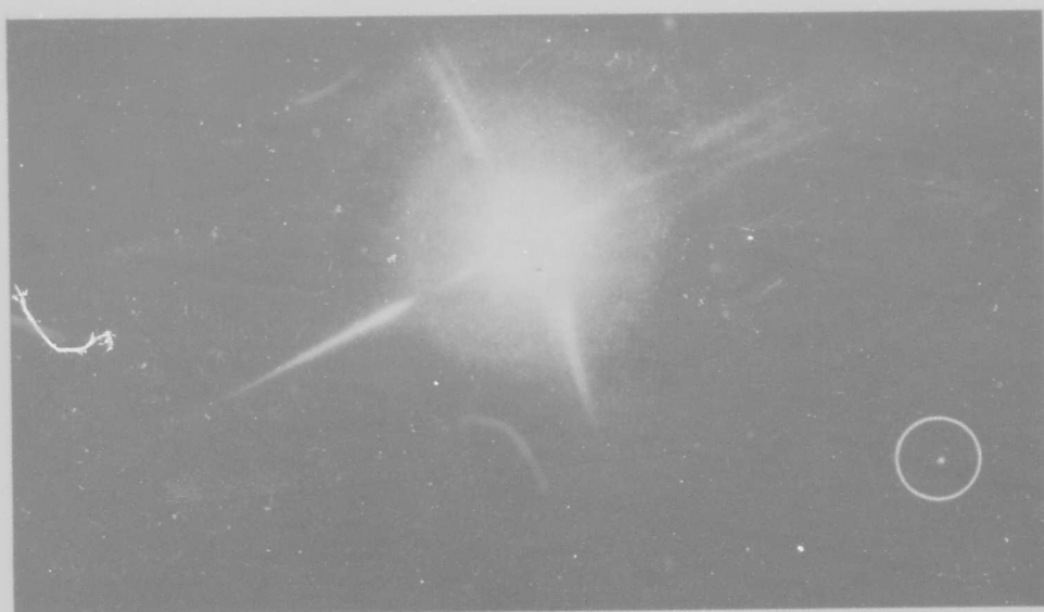
Fig. 77 Thirty Minute Exposure, Projected Aperture Size 200 \text{ \AA} \times 200 \text{ \AA} . Only continuous halos are visible. Diffraction pattern shown at 2\times , image of aperture (circled) at 24,000\times . P1502
