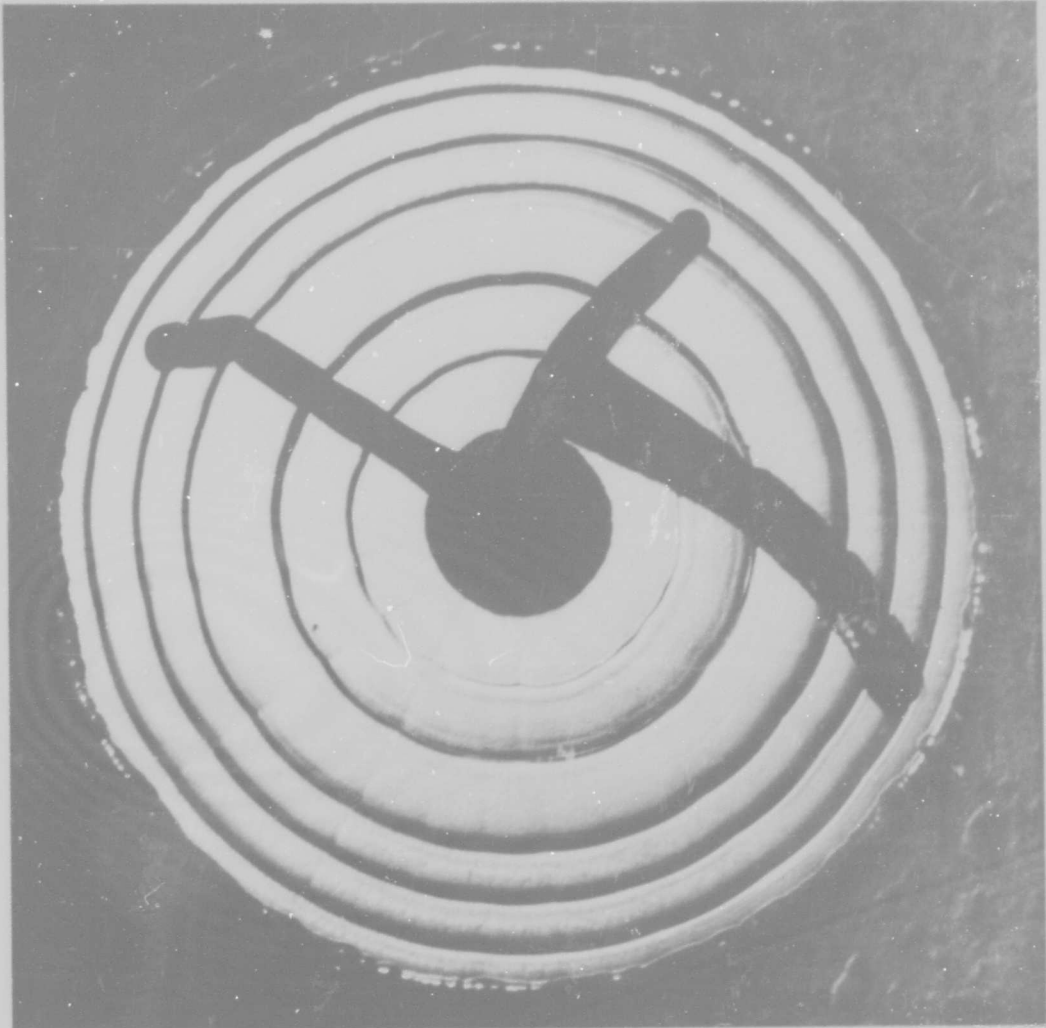
Fig. 17 Same Cross Section as Fig.16 Treated to Show Radial Lines Associated With Inner Nodules
