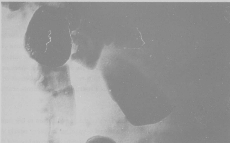
Fig. 61a High Magnification View of Crystalline Regions in Chemically Thinned Boron Filament. 92,000 \times . P1459-6a
