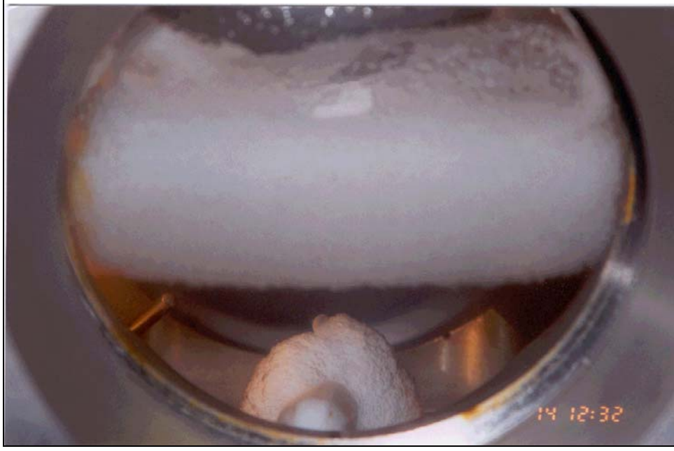
Gas Hydrate formed in Dynamic conditions
