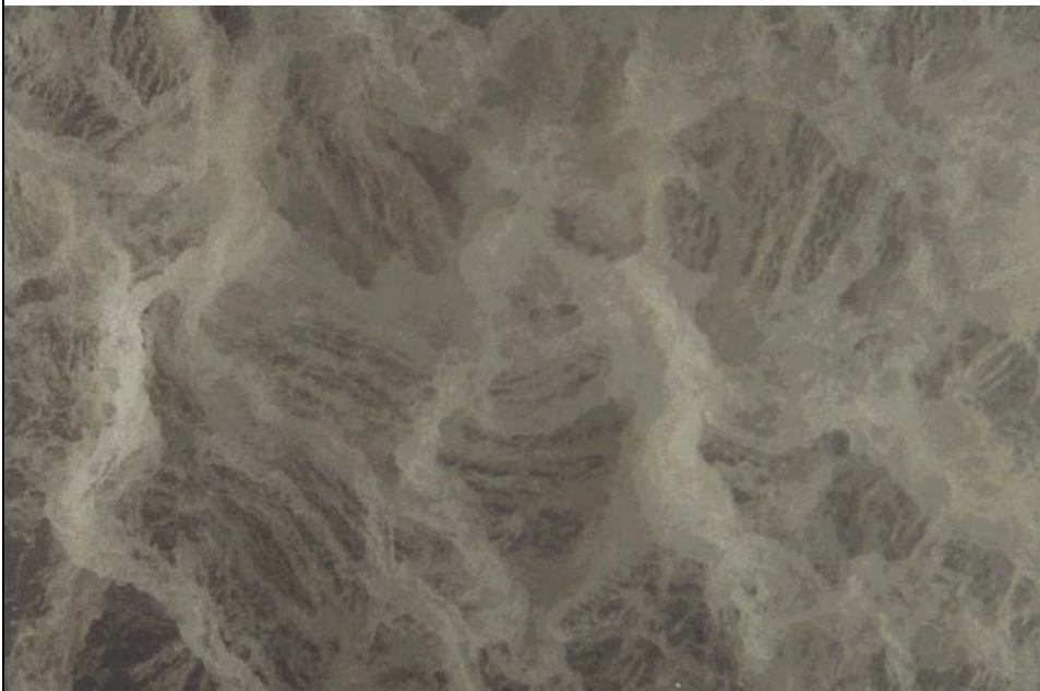
Gas Hydrate Crystals formed in Dynamic flow
