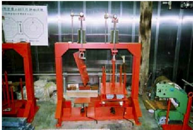
Compression Testing Apparatus (Static Loading Test)
