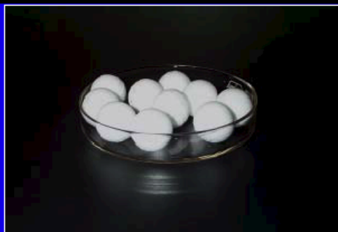
20mm in diameter NGH Pellets manufactured by Mitsui
