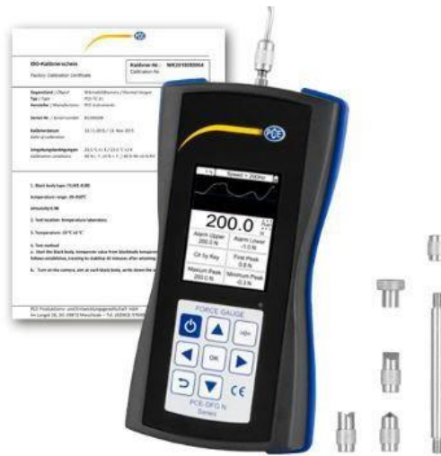
Figure 4. PCE Instruments digital force gauge N 200 with calibration certificate and attachments. The PCE Instruments digital force gauge possesses an internal storage option of 100 measured values and a USB interface available for data transmission. The PCE Instruments Digital Force gauge also has a 1600 Hz sampling rate and a graphical analysis display included.
