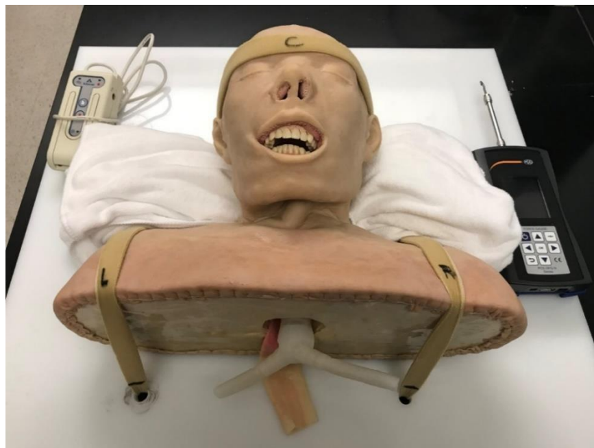
Figure 8. Test Platform Configuration. The test platform is pictured above in the evaluation configuration with the digital force gauge and a pressure mapping receiver.
