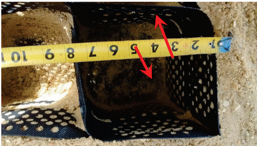
Figure 6-4. Buckling of the cell wall of the 8-in.-thick geocells after completion of Phase 2 trafficking.
