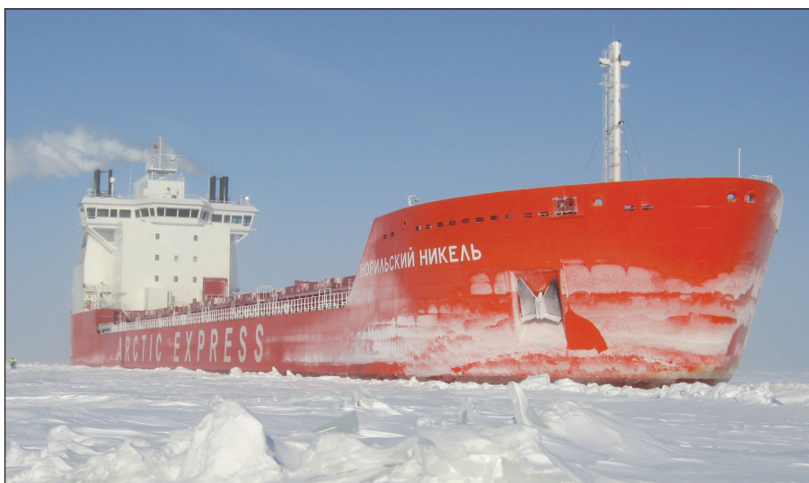
Icebreaking container ship Norilsk Nickel that routinely sails from the port of Dudinka carrying finished metals of the company Nornickel. (Aker Arctic)
