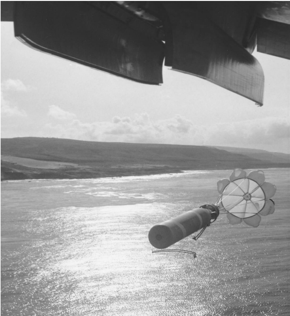
Air-drop test of a Mark 46 torpedo from an ASW aircraft off San Clemente Island to ensure proper break-away of restraining clamps and parachute deployment.
