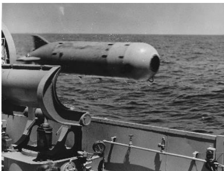
Immediate post-World War II torpedo efforts by NOTS Pasadena centered on the Mark 32 torpedo, development of which had begun during the war. The top figure is a representation of the torpedo's programmed search technique. Left photo shows siderail launch of the weapon.
