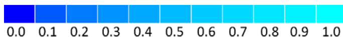
Figure 7. Shades of blue based on 1 part blue plus 0 to 1 part green in steps of 0.1. The left color patch is (0, 0, 255) and rightmost patch is (0, 255, 255). Steps in between 0.0 and 1.0 represent the amount of green that is added to one part of blue. Chart is calibrated for displays with a gamma of 2.2.
