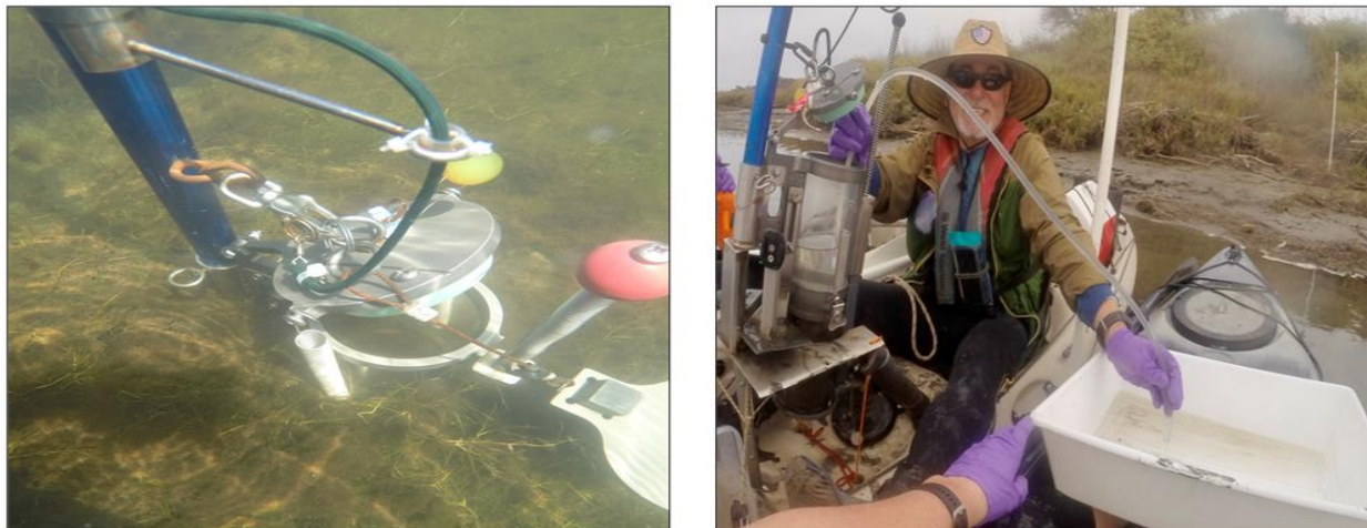
Figure 4 Subsamplers/ BCA sample collection. The SUBS sampler in water just prior to collecting sample (left). Suction tube method of draining water, in this case into tray for benthic sample collection (right).
