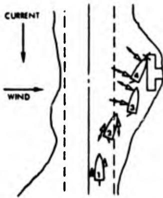
Fig. 4 Typical casualty that occurred when a vessel was unable to maintain its heading
