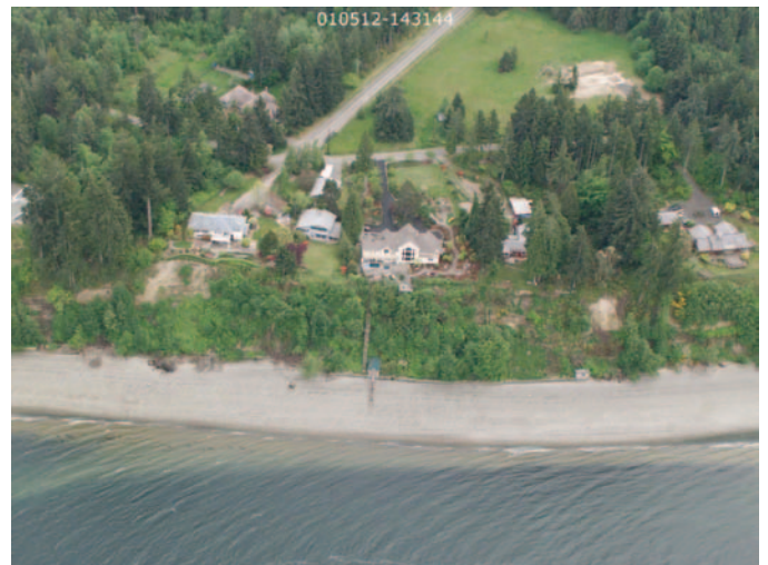
Figure 12. Homes built along the top edge of a bluff in southern Puget Sound. Setback requirements vary among jurisdictions. The desire for views typically leads property owners to build as close to the bluff as regulations allow.
