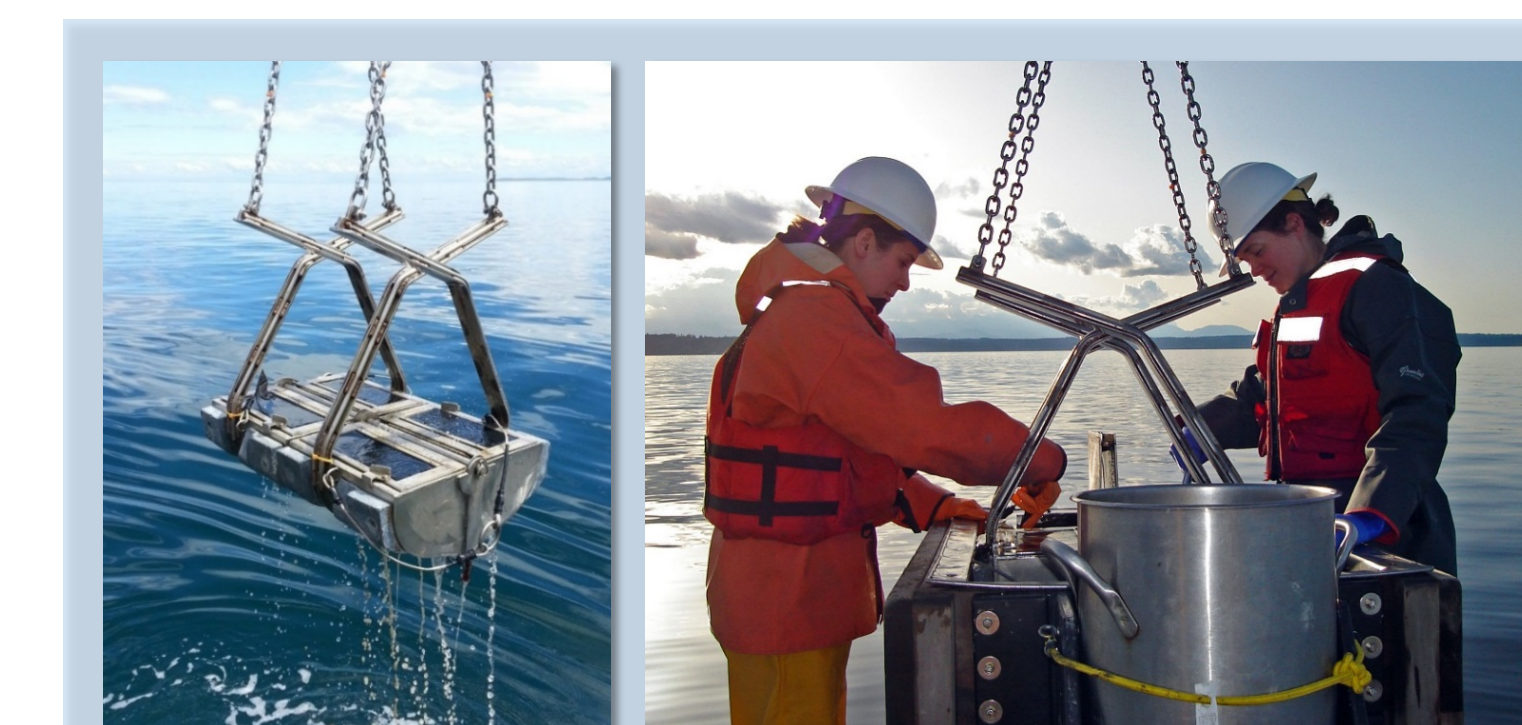
Sediment is collected using a double van Veen grab.
